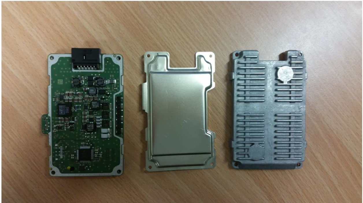
Main Board with Shielding and Cooling Element
