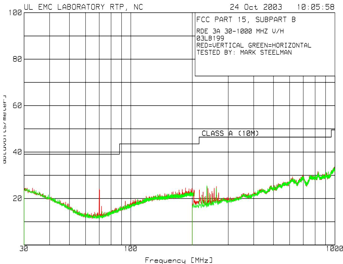
**Test 3, Item A - Discrete Data:** Radiated Disturbance Emissions - 30 MHz to 1000 MHz
