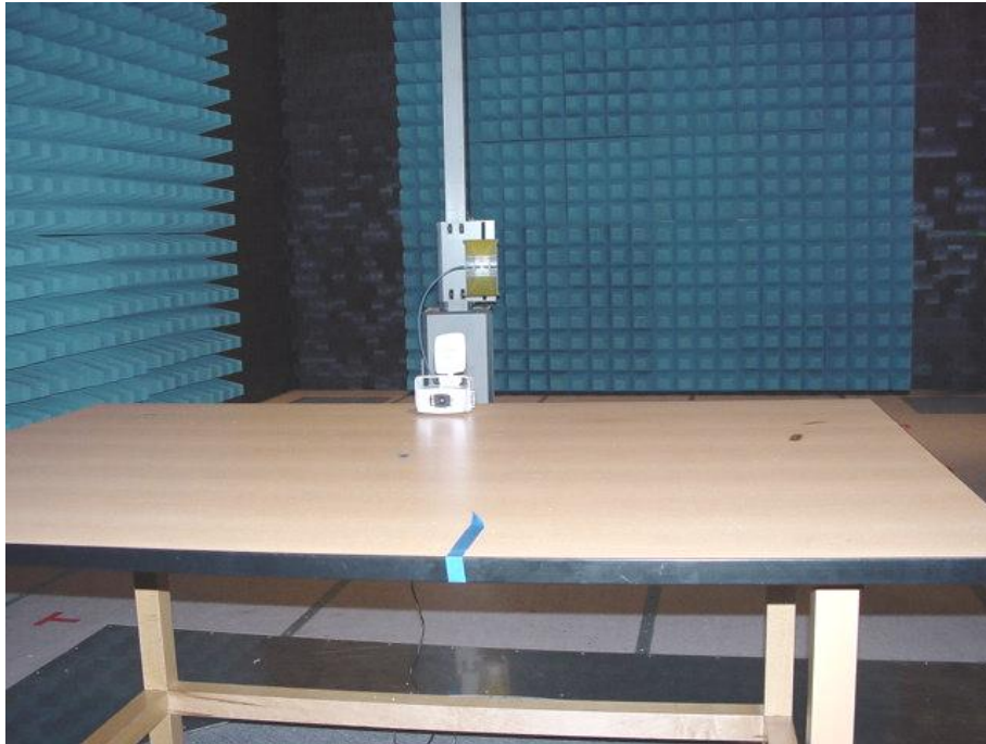
Photo3 Test Setup for Radiated Disturbance Test
