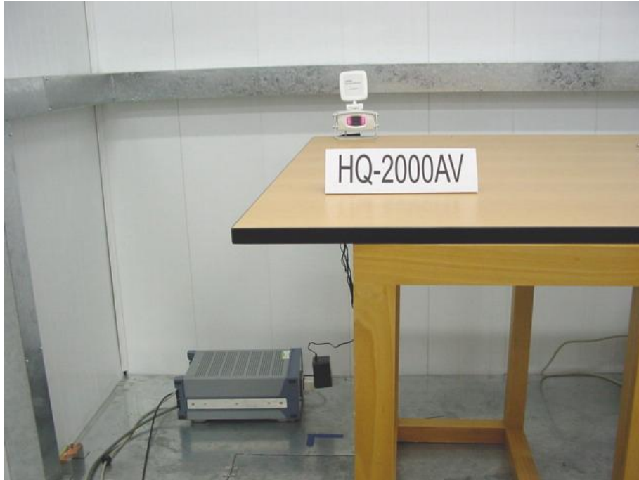
Photo 1 Test Setup for Conducted Disturbance Test
