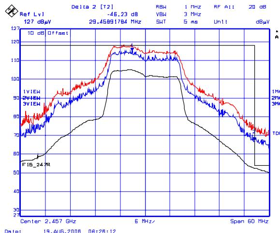
**Plot 23(b): Lower Band-Edge Transmitter Radiated Emissions @ 3 Meters, Vertical Polarization**
