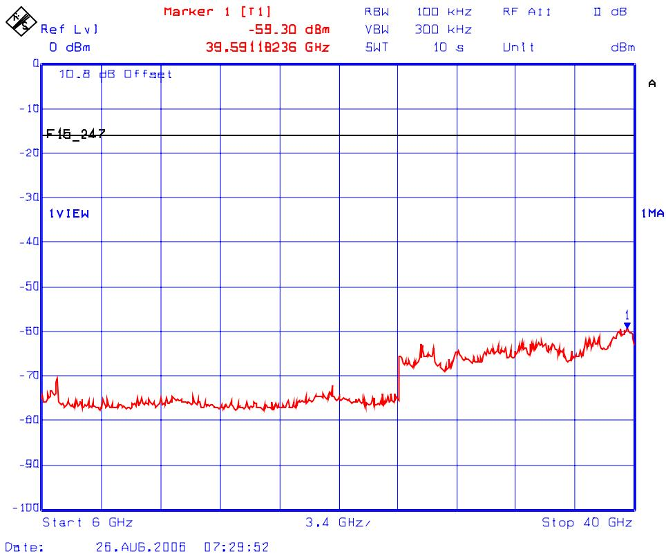
**Plot #40(a): Conducted Spurious Emissions & Intermodulation with 2 RF Output Signals on Antenna Port A (2447 MHz, Setting 20.0dBm and 5220 MHz Setting 17.0dBm)**
