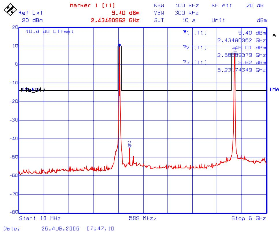
**Plot #40(b): Conducted Spurious Emissions & Intermodulation with 2 RF Output Signals on Antenna Port A (2447 MHz, Setting 20.0dBm and 5220 MHz Setting 17.0dBm)**
