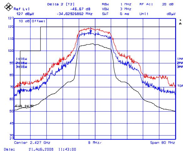
**Plot 4(b): Lower Band-Edge Transmitter Radiated Emissions @ 3 Meters, Vertical Polarization**
