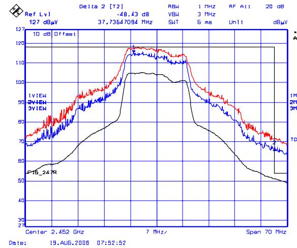
**Plot 22(b): Lower Band-Edge Transmitter Radiated Emissions @ 3 Meters, Vertical Polarization**
