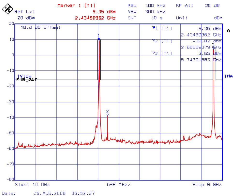
**Plot #42(b): Conducted Spurious Emissions & Intermodulation with 2 RF Output Signals on Antenna Port A (2447 MHz, Setting 20.0dBm and 5745 MHz Setting 15.0dBm)**
