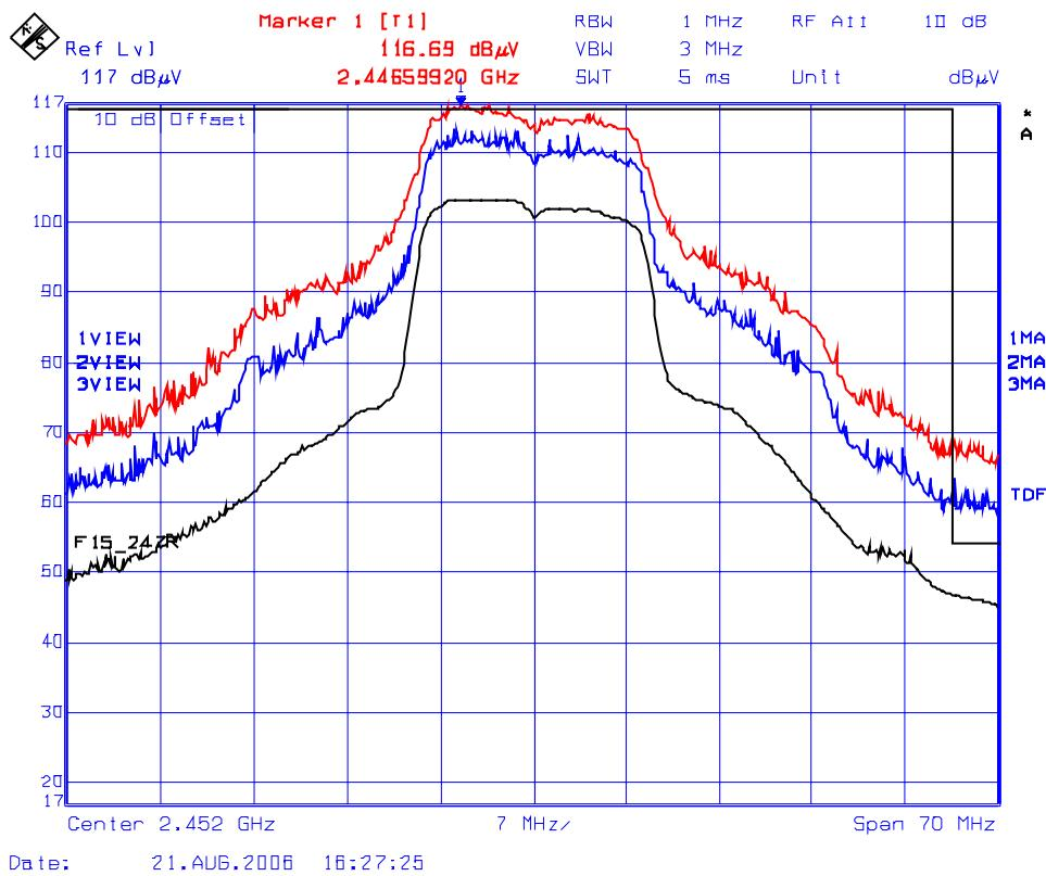
**Plot 10(a): Lower Band-Edge Transmitter Radiated Emissions @ 3 Meters, Horizontal Polarization**
