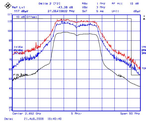
**Plot 12(a): Lower Band-Edge Transmitter Radiated Emissions @ 3 Meters, Horizontal Polarization**
