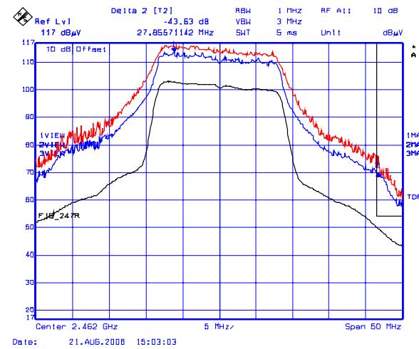
**Plot 11(b): Lower Band-Edge Transmitter Radiated Emissions @ 3 Meters, Vertical Polarization**
