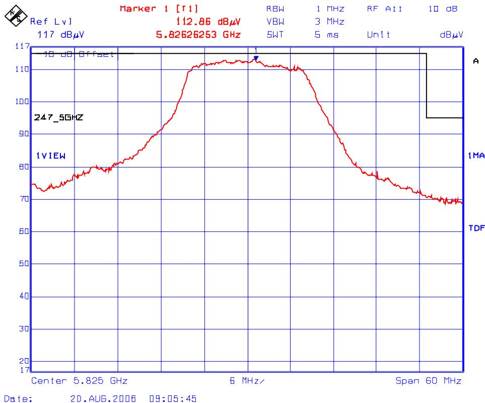
**Plot 26(b): Lower Band-Edge Transmitter Radiated Emissions @ 3 Meters, Vertical Horizontal**
