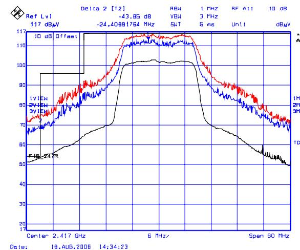
**Plot 15(b): Lower Band-Edge Transmitter Radiated Emissions @ 3 Meters, Vertical Polarization**
