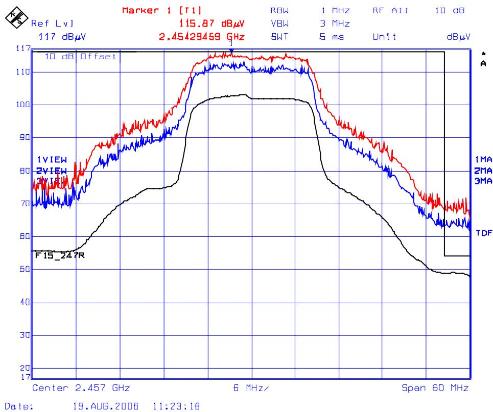
**Plot 24(a): Lower Band-Edge Transmitter Radiated Emissions @ 3 Meters, Horizontal Polarization**
