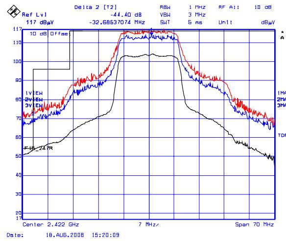
**Plot 16(b): Lower Band-Edge Transmitter Radiated Emissions @ 3 Meters, Vertical Polarization**
