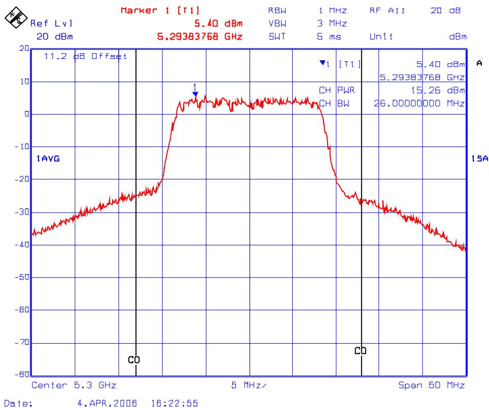
**Plot #32: Channel Conducted Power in 26 dB Bandwidth**
