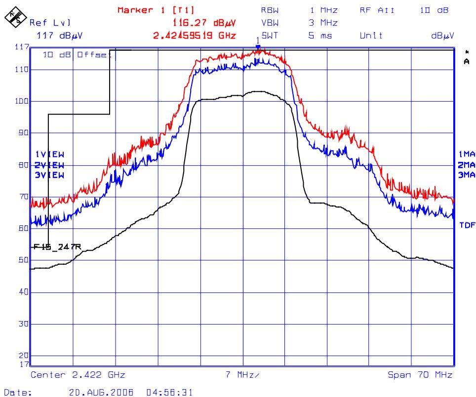
**Plot 17(a): Lower Band-Edge Transmitter Radiated Emissions @ 3 Meters, Horizontal Polarization**
