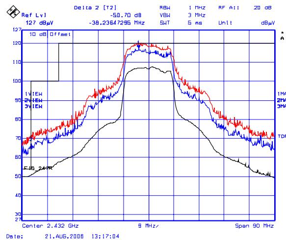
**Plot 5(b): Lower Band-Edge Transmitter Radiated Emissions @ 3 Meters, Vertical Polarization**
