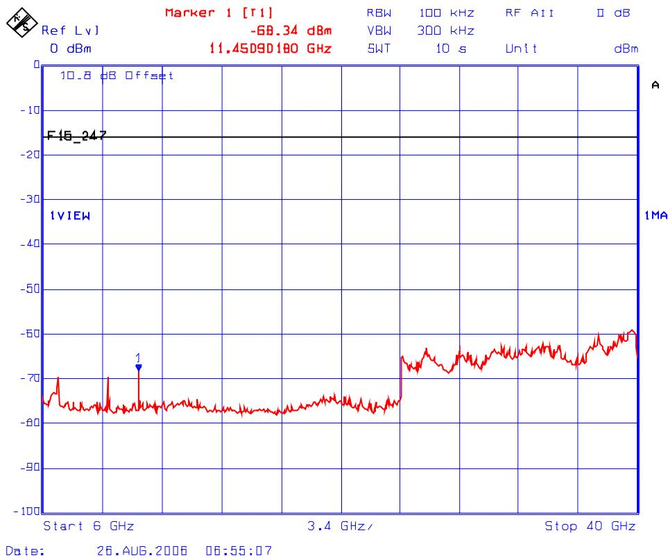
**Plot #43(a): Conducted Spurious Emissions & Intermodulation with 2 RF Output Signals on Antenna Port A (2447 MHz, Setting 20.0dBm and 5220 MHz Setting 17.0dBm)**
