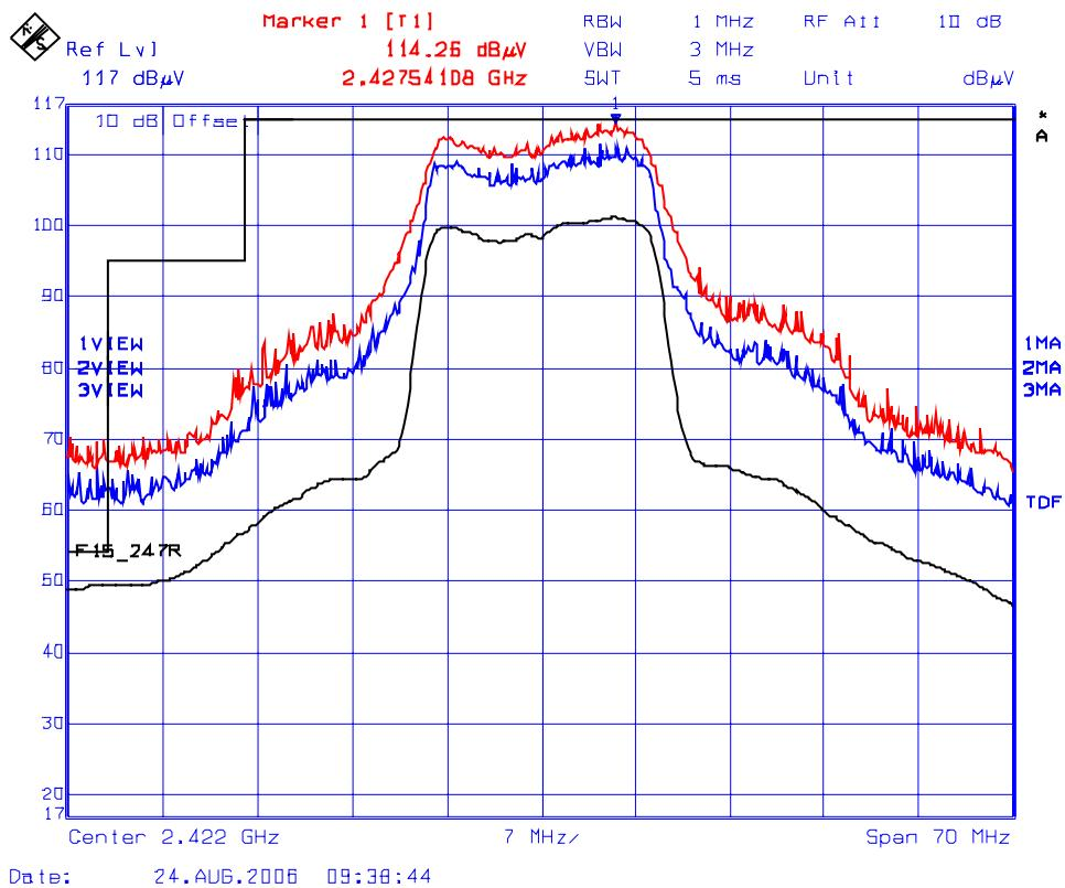
**Plot 4(a): Lower Band-Edge Transmitter Radiated Emissions @ 3 Meters, Horizontal Polarization**
