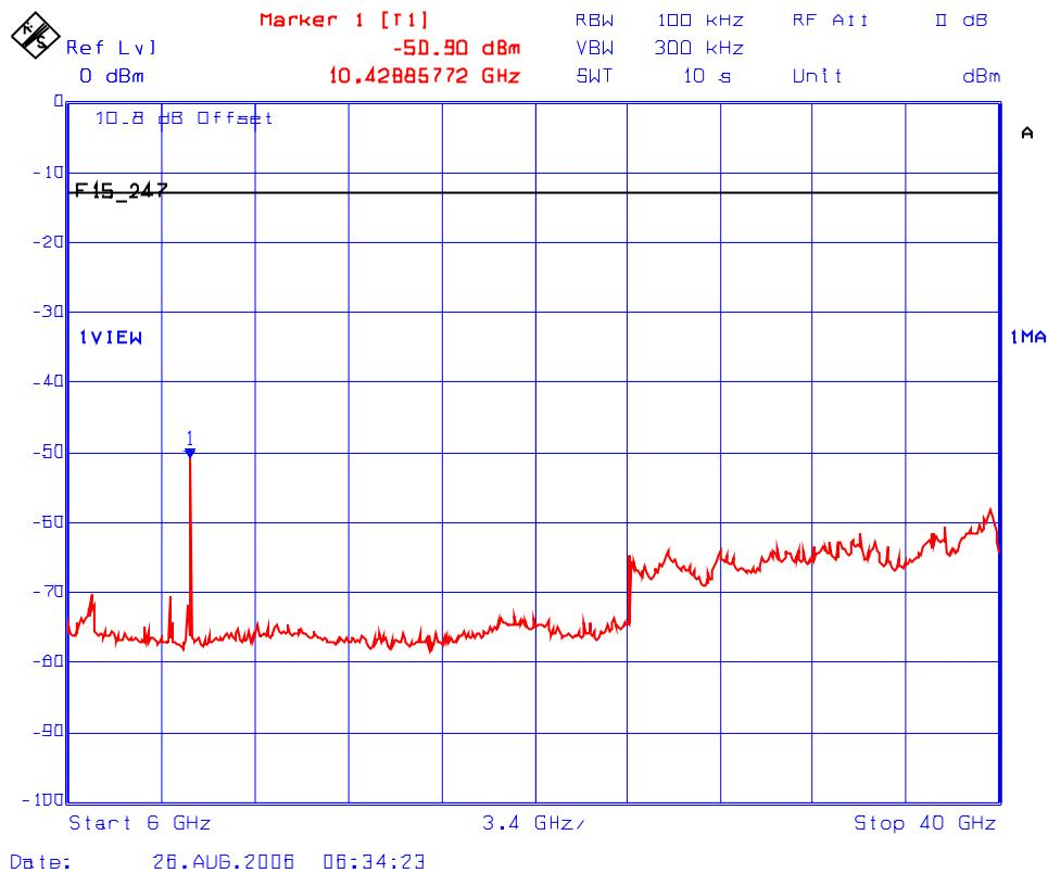
**Plot #44(a): Conducted Spurious Emissions & Intermodulation with 2 RF Output Signals on Antenna Port A (2447 MHz, Setting 20.0dBm and 5330 MHz Setting 18.0dBm)**
