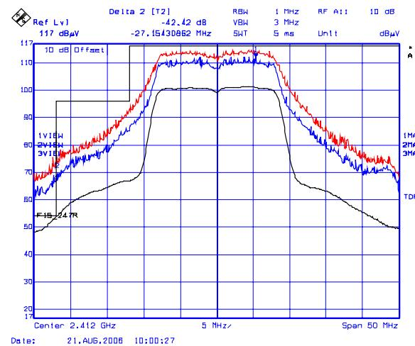
**Plot 1(b): Lower Band-Edge Transmitter Radiated Emissions @ 3 Meters, Vertical Polarization**
