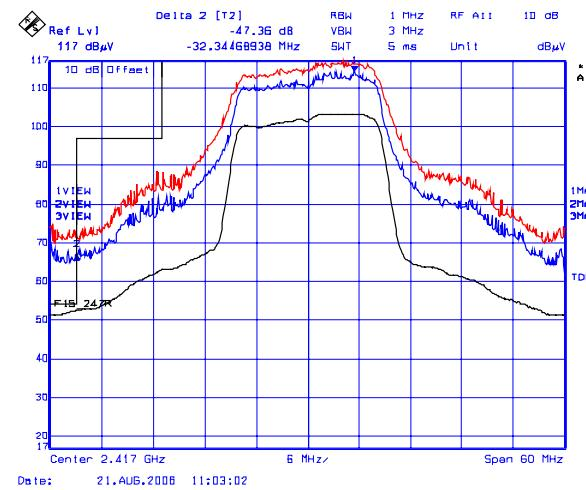
**Plot 2(b): Lower Band-Edge Transmitter Radiated Emissions @ 3 Meters, Vertical Polarization**
