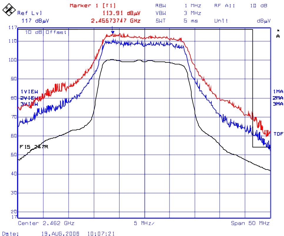
**Plot 25(a): Lower Band-Edge Transmitter Radiated Emissions @ 3 Meters, Horizontal Polarization**
