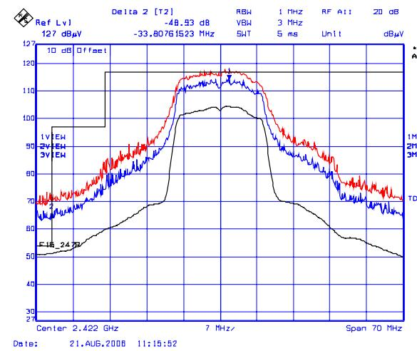
**Plot 3(b): Lower Band-Edge Transmitter Radiated Emissions @ 3 Meters, Vertical Polarization**
