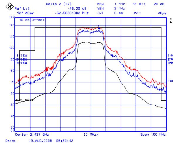
**Plot 19(b): Lower Band-Edge Transmitter Radiated Emissions @ 3 Meters, Vertical Polarization**
