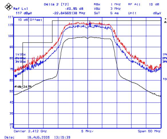
**Plot 14(b): Lower Band-Edge Transmitter Radiated Emissions @ 3 Meters, Vertical Polarization**
