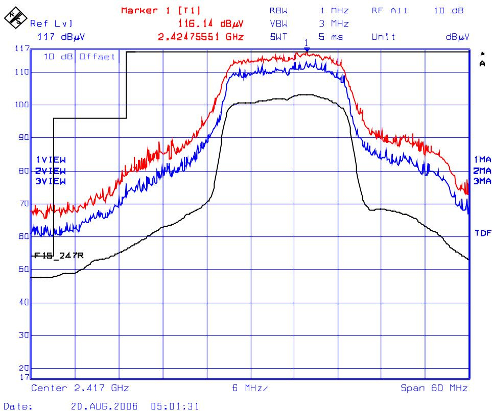
**Plot 16(a): Lower Band-Edge Transmitter Radiated Emissions @ 3 Meters, Horizontal Polarization**
