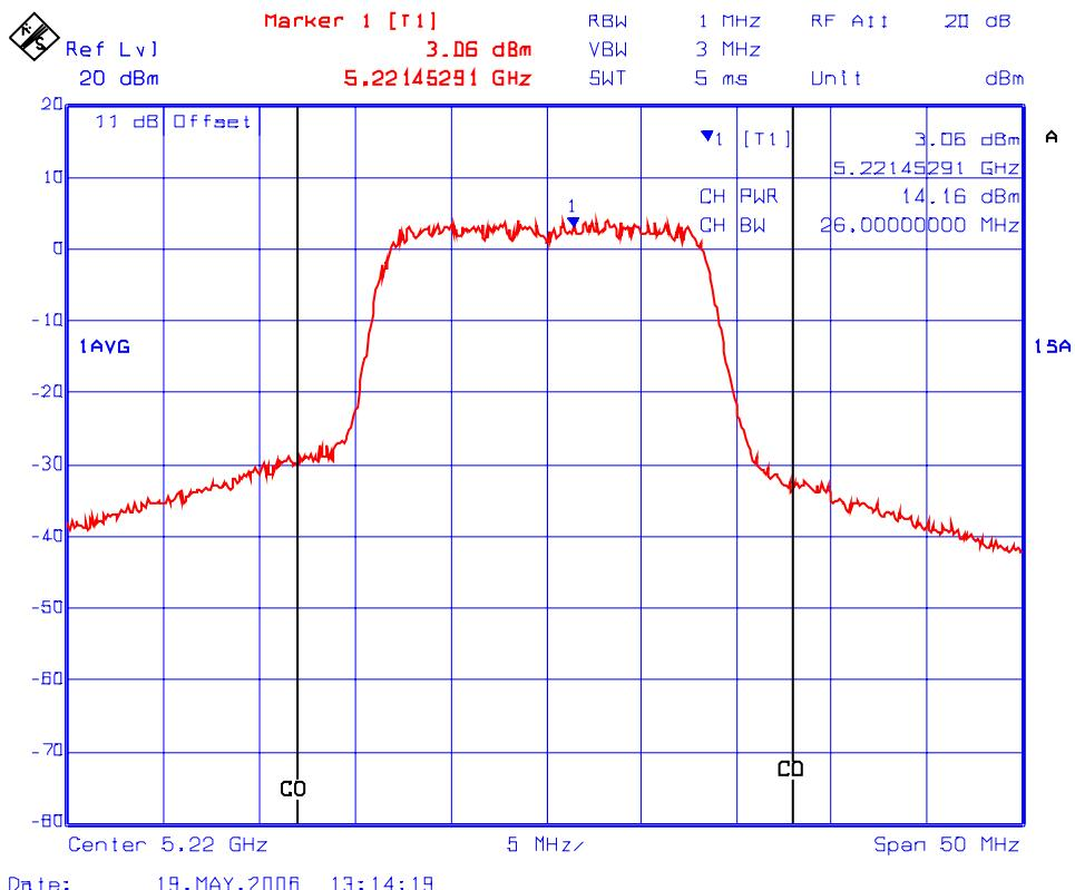
**Plot #35: Channel Conducted Power in 26 dB Bandwidth**
