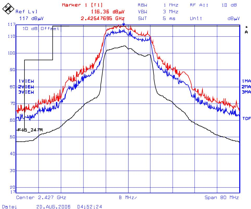
**Plot 18(a): Lower Band-Edge Transmitter Radiated Emissions @ 3 Meters, Horizontal Polarization**
