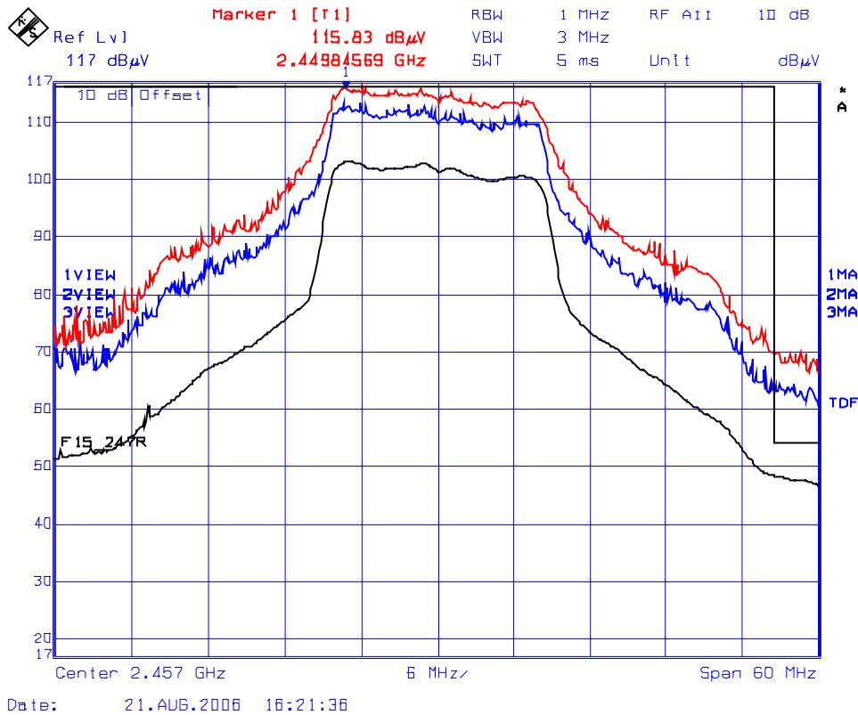
**Plot 11(a): Lower Band-Edge Transmitter Radiated Emissions @ 3 Meters, Horizontal Polarization**
