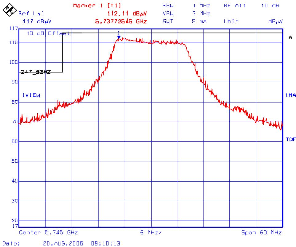
**Plot 25(b): Lower Band-Edge Transmitter Radiated Emissions @ 3 Meters, Vertical Horizontal**
