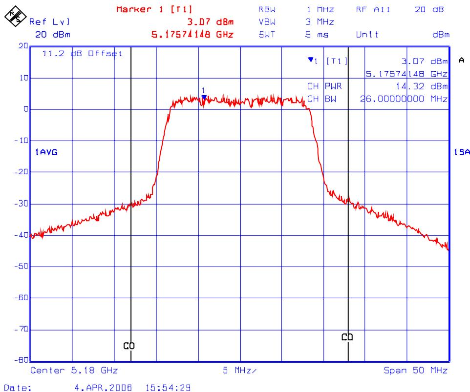
**Plot #28: Channel Conducted Power in 26 dB Bandwidth**
