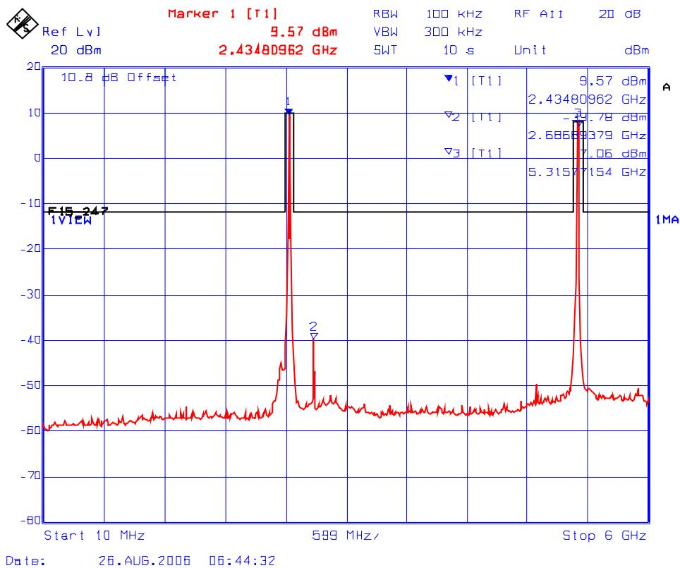
**Plot #44(b): Conducted Spurious Emissions & Intermodulation with 2 RF Output Signals on Antenna Port A (2447 MHz, Setting 20.0dBm and 5330 MHz Setting 18.0dBm)**
