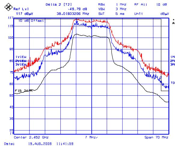
**Plot 23(a): Lower Band-Edge Transmitter Radiated Emissions @ 3 Meters, Horizontal Polarization**
