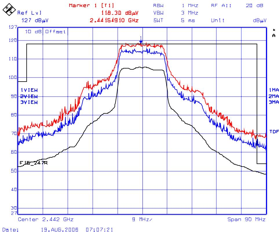
**Plot 20(b): Lower Band-Edge Transmitter Radiated Emissions @ 3 Meters, Vertical Polarization**
