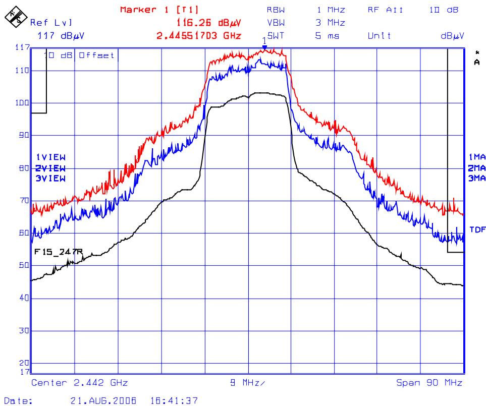
**Plot 8(a): Lower Band-Edge Transmitter Radiated Emissions @ 3 Meters, Horizontal Polarization**
