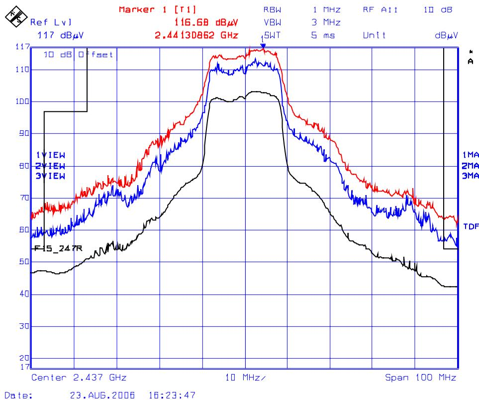
**Plot 7(a): Lower Band-Edge Transmitter Radiated Emissions @ 3 Meters, Horizontal Polarization**
