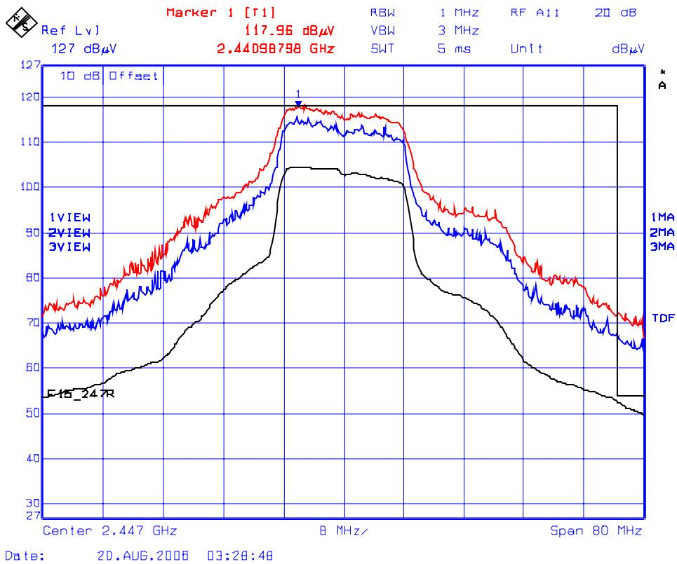
**Plot 22(a): Lower Band-Edge Transmitter Radiated Emissions @ 3 Meters, Horizontal Polarization**
