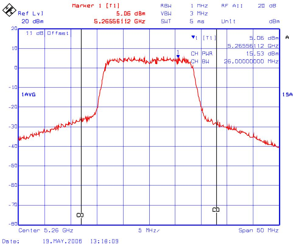
**Plot #37: Channel Conducted Power in 26 dB Bandwidth**
