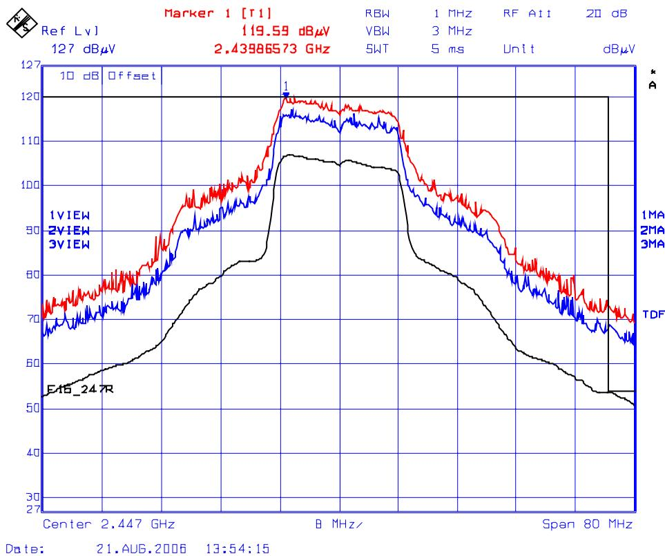
**Plot 8(b): Lower Band-Edge Transmitter Radiated Emissions @ 3 Meters, Vertical Polarization**
