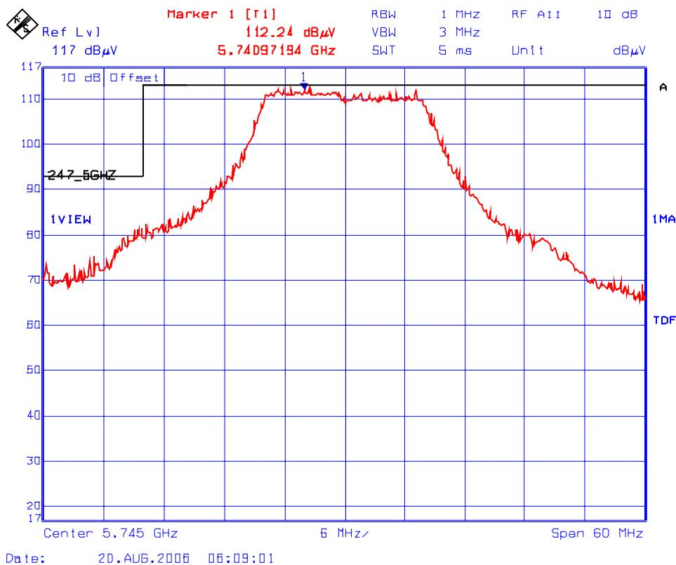
**Plot 26(a): Lower Band-Edge Transmitter Radiated Emissions @ 3 Meters, Horizontal Polarization**
