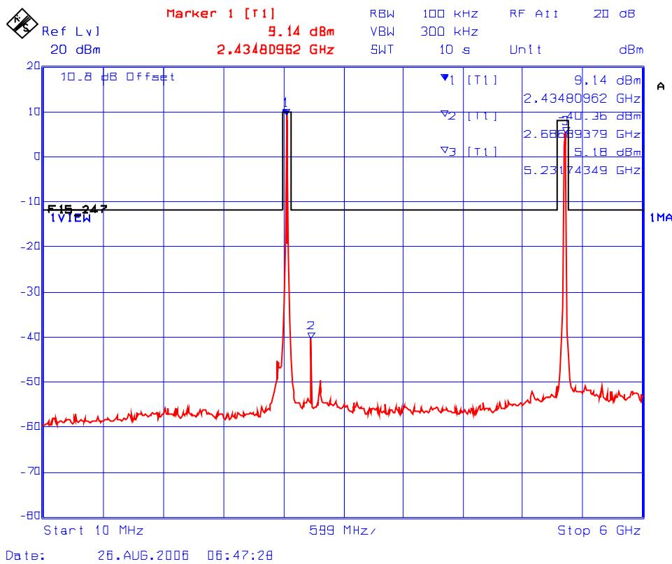
**Plot #43(b): Conducted Spurious Emissions & Intermodulation with 2 RF Output Signals on Antenna Port A (2447 MHz, Setting 20.0dBm and 5220 MHz Setting 17.0dBm)**
