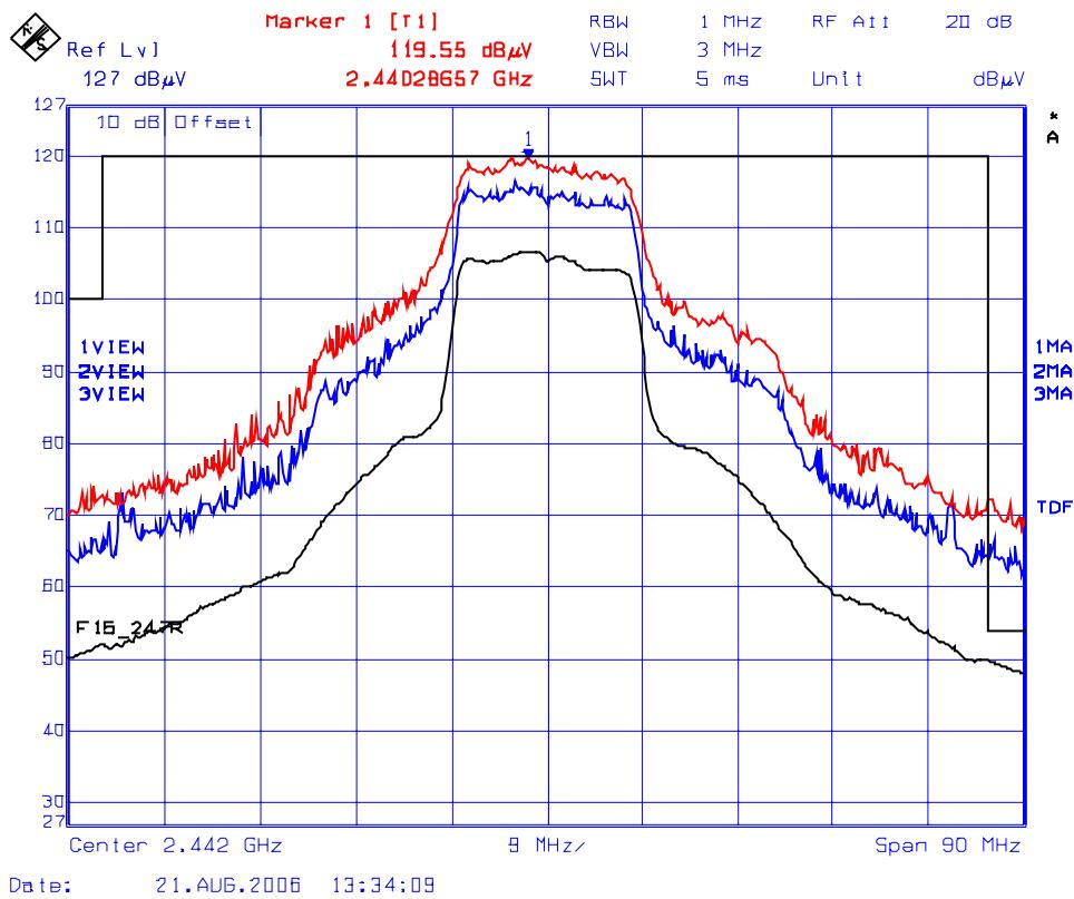
**Plot 7(b): Lower Band-Edge Transmitter Radiated Emissions @ 3 Meters, Vertical Polarization**
