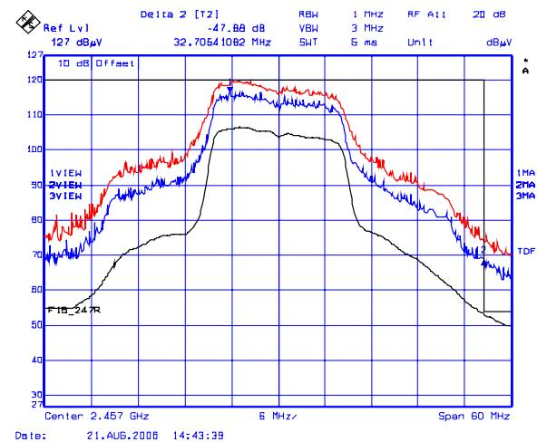
**Plot 10(b): Lower Band-Edge Transmitter Radiated Emissions @ 3 Meters, Vertical Polarization**
