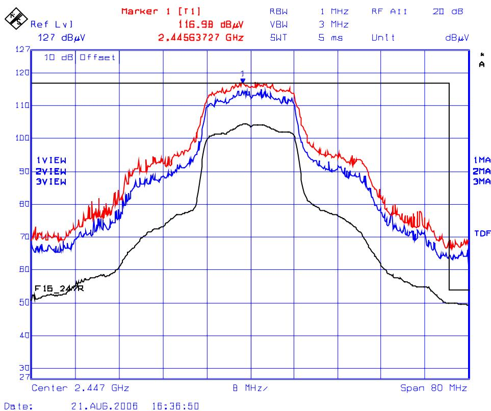
**Plot 9(a): Lower Band-Edge Transmitter Radiated Emissions @ 3 Meters, Horizontal Polarization**
