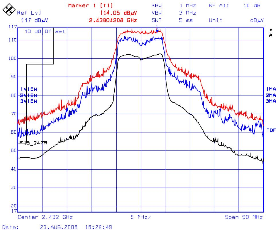
**Plot 6(a): Lower Band-Edge Transmitter Radiated Emissions @ 3 Meters, Horizontal Polarization**
