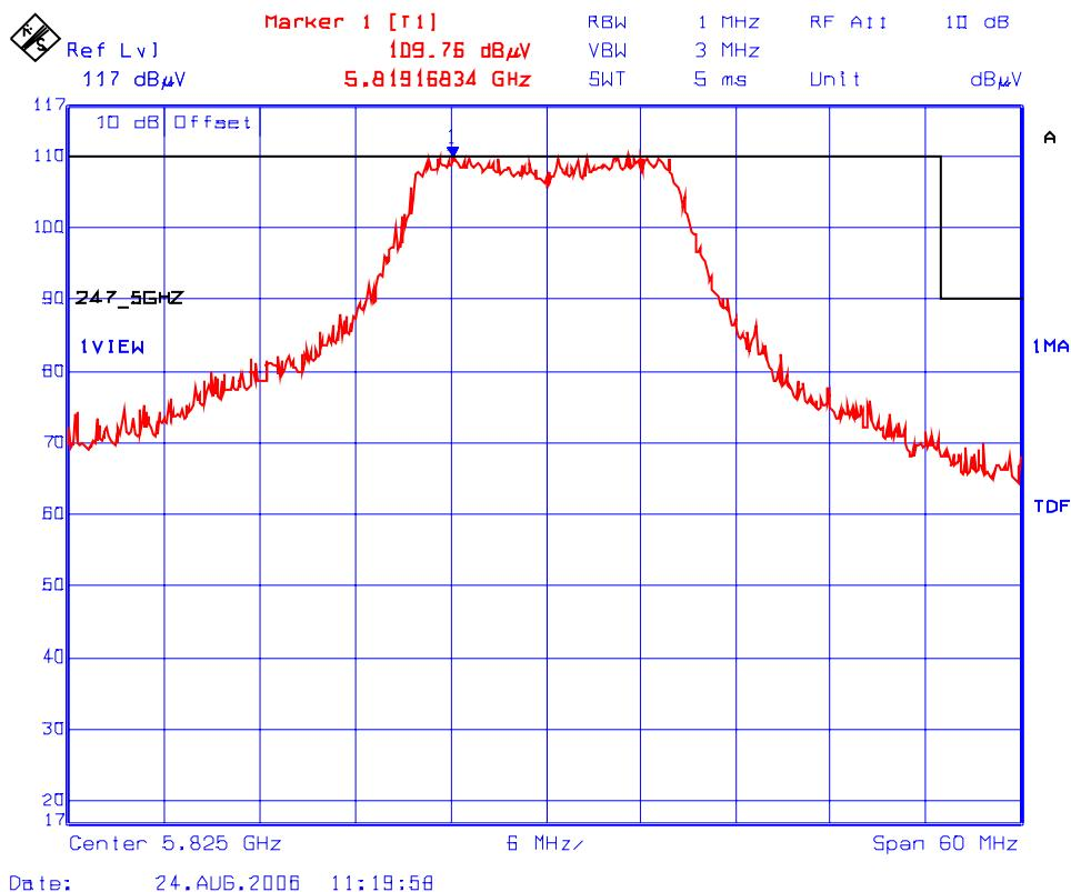
**Plot 13(b): Lower Band-Edge Transmitter Radiated Emissions @ 3 Meters, Vertical Horizontal**
