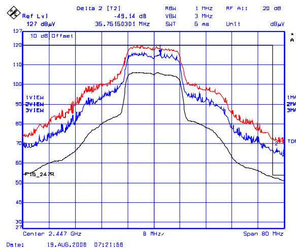
**Plot 21(b): Lower Band-Edge Transmitter Radiated Emissions @ 3 Meters, Vertical Polarization**
