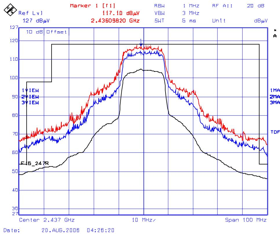
**Plot 20(a): Lower Band-Edge Transmitter Radiated Emissions @ 3 Meters, Horizontal Polarization**
