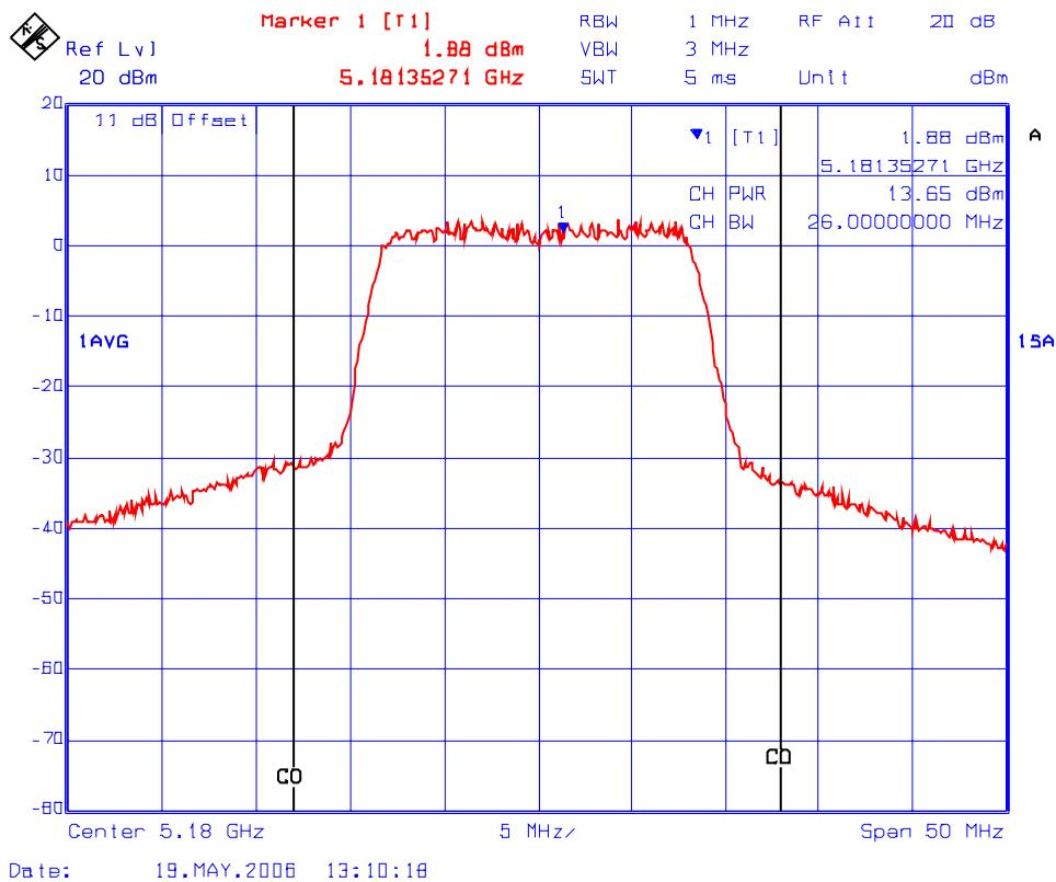
**Plot #34: Channel Conducted Power in 26 dB Bandwidth**
