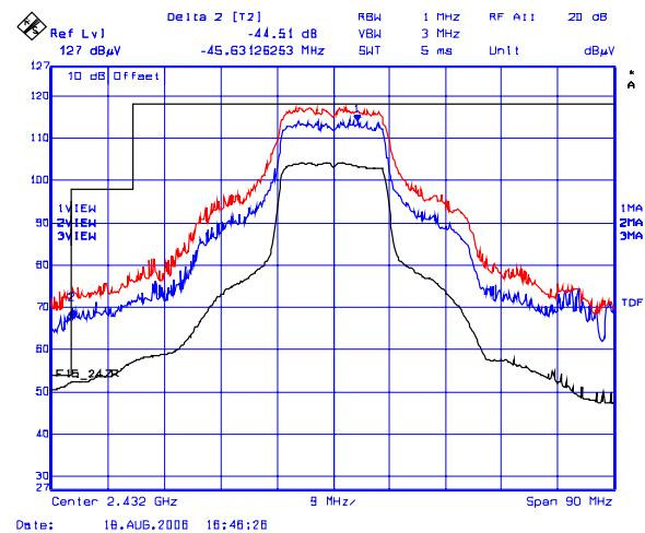
**Plot 18(b): Lower Band-Edge Transmitter Radiated Emissions @ 3 Meters, Vertical Polarization**
