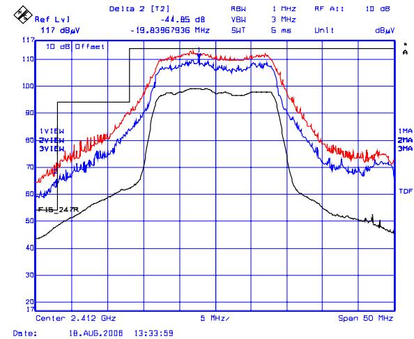
**Plot 15(a): Lower Band-Edge Transmitter Radiated Emissions @ 3 Meters, Horizontal Polarization**
