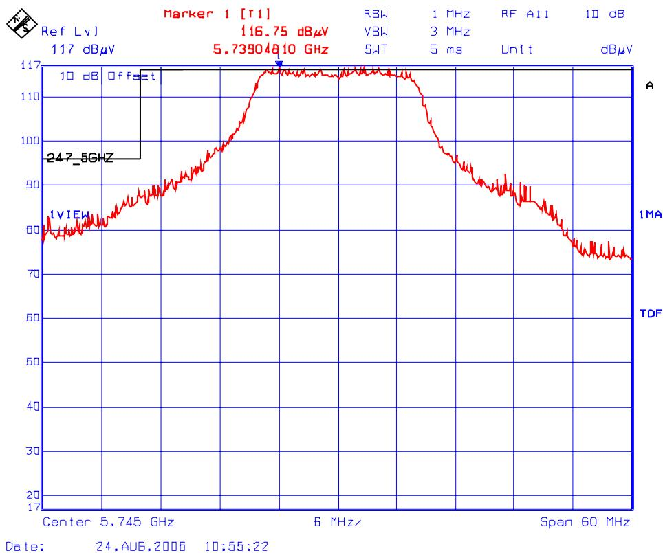
**Plot 13(a): Lower Band-Edge Transmitter Radiated Emissions @ 3 Meters, Horizontal Polarization**
