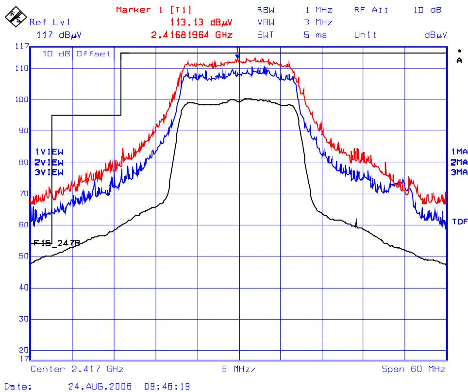
**Plot 3(a): Lower Band-Edge Transmitter Radiated Emissions @ 3 Meters, Horizontal Polarization**
