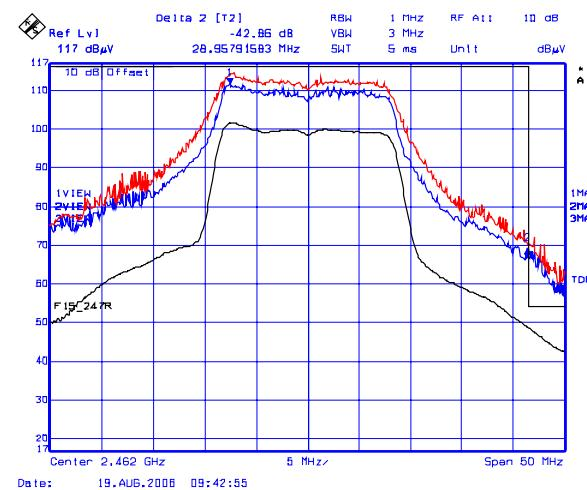
**Plot 24(b): Lower Band-Edge Transmitter Radiated Emissions @ 3 Meters, Vertical Polarization**
