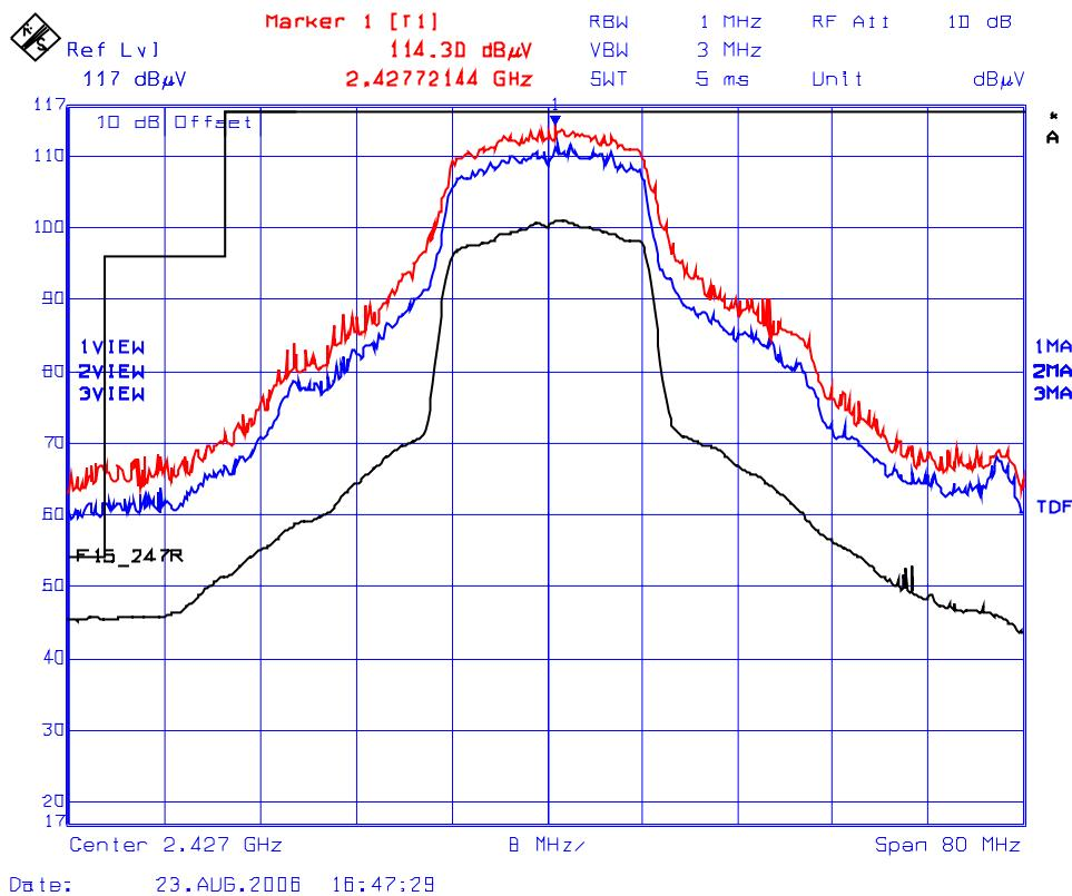
**Plot 5(a): Lower Band-Edge Transmitter Radiated Emissions @ 3 Meters, Horizontal Polarization**
