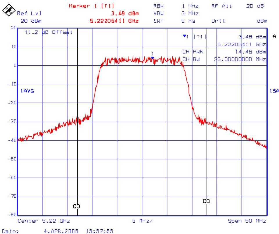
**Plot #29: Channel Conducted Power in 26 dB Bandwidth**
