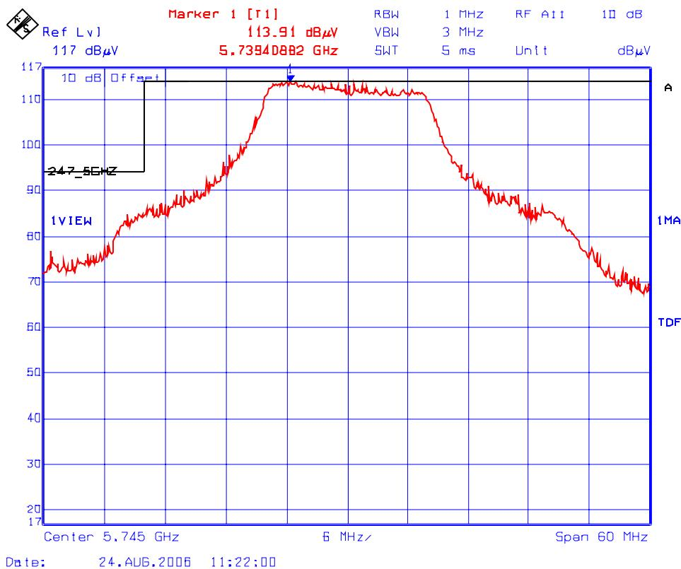
**Plot 12(b): Lower Band-Edge Transmitter Radiated Emissions @ 3 Meters, Vertical Horizontal**
