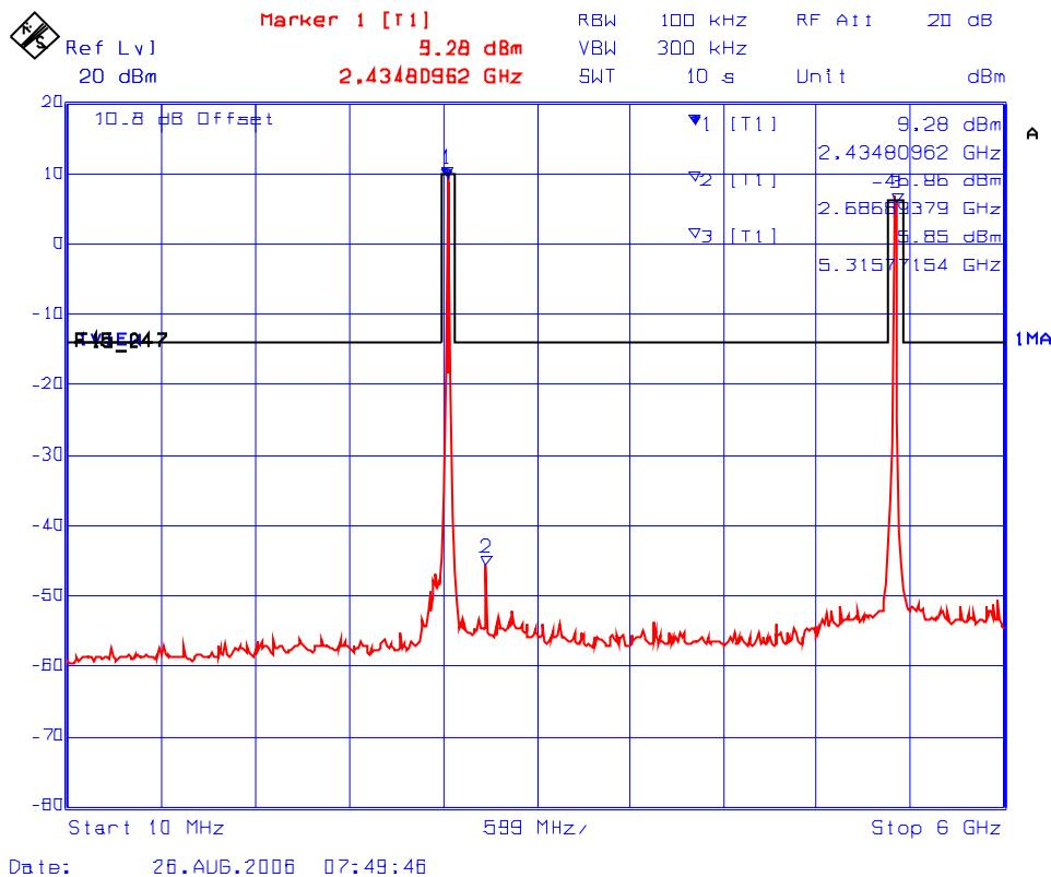
**Plot #41(b): Conducted Spurious Emissions & Intermodulation with 2 RF Output Signals on Antenna Port A (2447 MHz, Setting 20.0dBm and 5330 MHz Setting 18.0dBm)**
