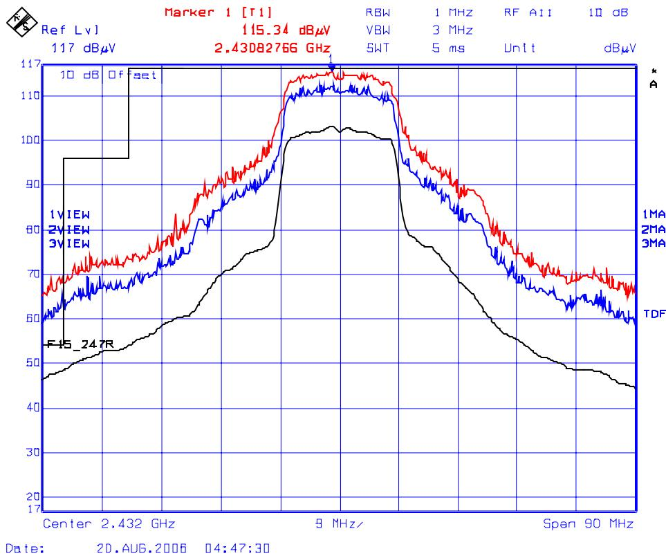
**Plot 19(a): Lower Band-Edge Transmitter Radiated Emissions @ 3 Meters, Horizontal Polarization**
