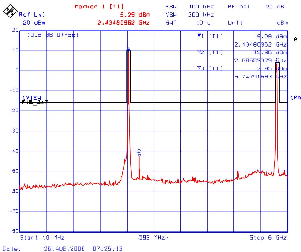
**Plot #39(b): Conducted Spurious Emissions & Intermodulation with 2 RF Output Signals on Antenna Port A (2447 MHz, Setting 20.0dBm and 5745 MHz Setting 15.0dBm)**
