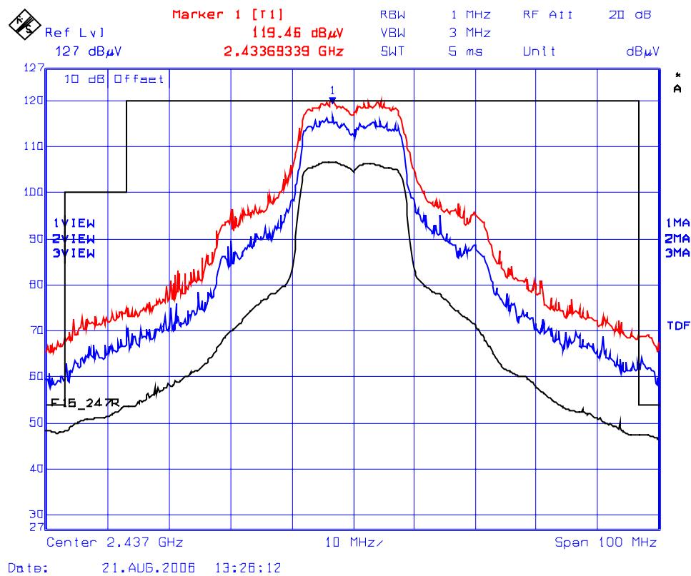
**Plot 6(b): Lower Band-Edge Transmitter Radiated Emissions @ 3 Meters, Vertical Polarization**
