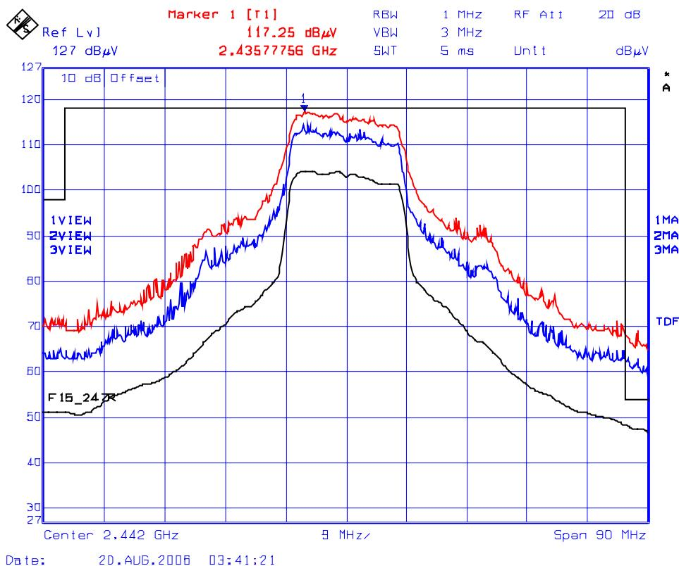
**Plot 21(a): Lower Band-Edge Transmitter Radiated Emissions @ 3 Meters, Horizontal Polarization**
