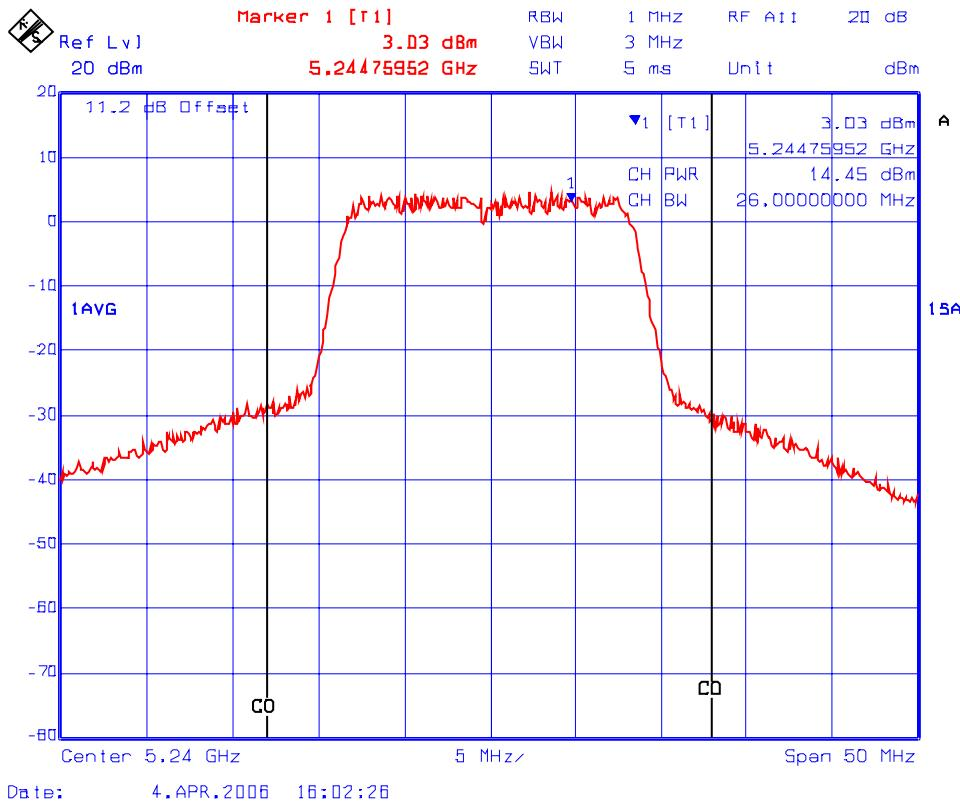
**Plot #30: Channel Conducted Power in 26 dB Bandwidth**
