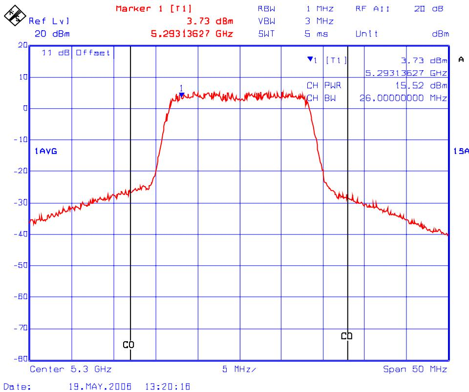
**Plot #38: Channel Conducted Power in 26 dB Bandwidth**
