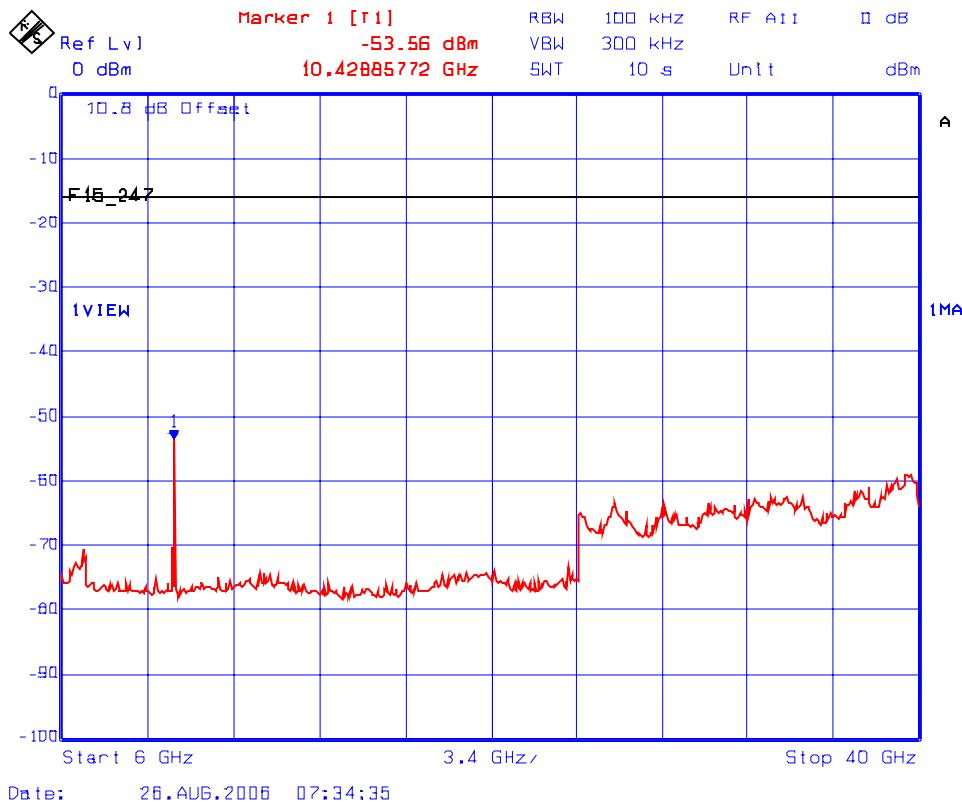
**Plot #41(a): Conducted Spurious Emissions & Intermodulation with 2 RF Output Signals on Antenna Port A (2447 MHz, Setting 20.0dBm and 5330 MHz Setting 18.0dBm)**
