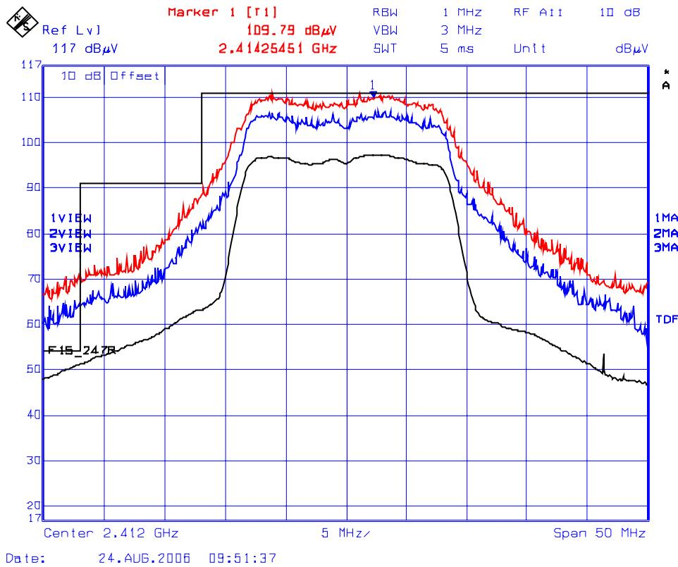
**Plot 2(a): Lower Band-Edge Transmitter Radiated Emissions @ 3 Meters, Horizontal Polarization**
