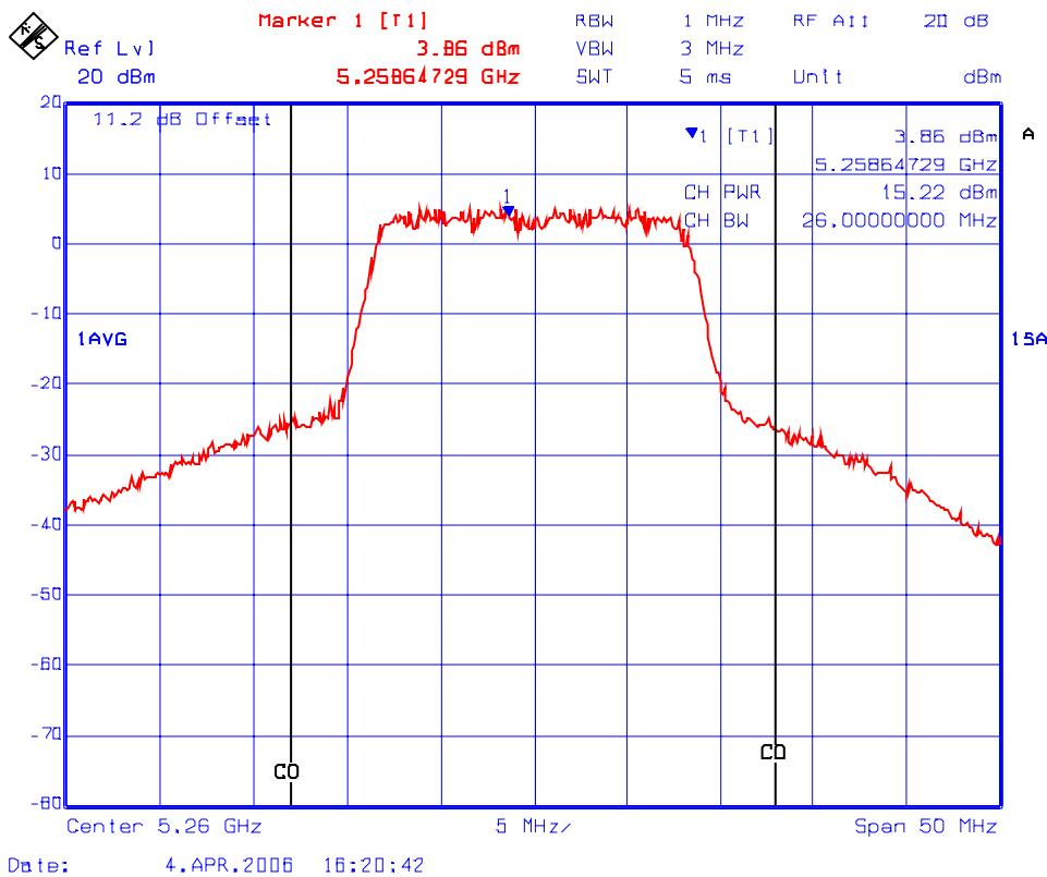
**Plot #31: Channel Conducted Power in 26 dB Bandwidth**
