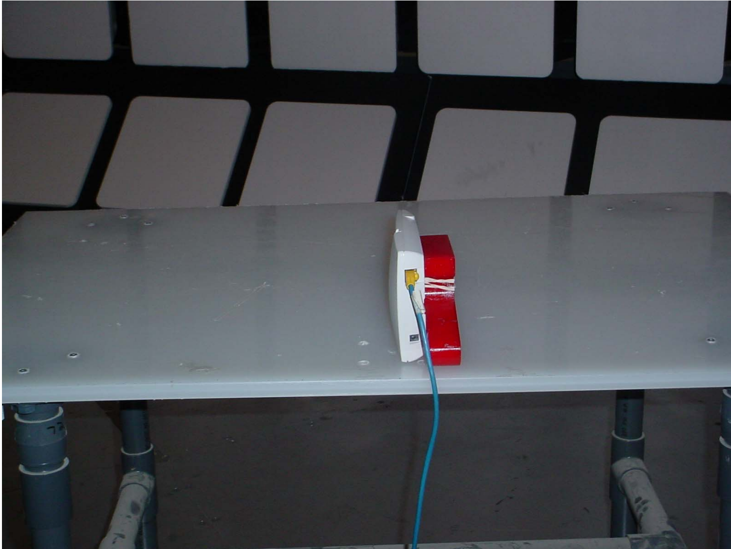
Photo #4: Altitude 350-2 Access Point with internal antennas – Test Orthogonal Position #2
