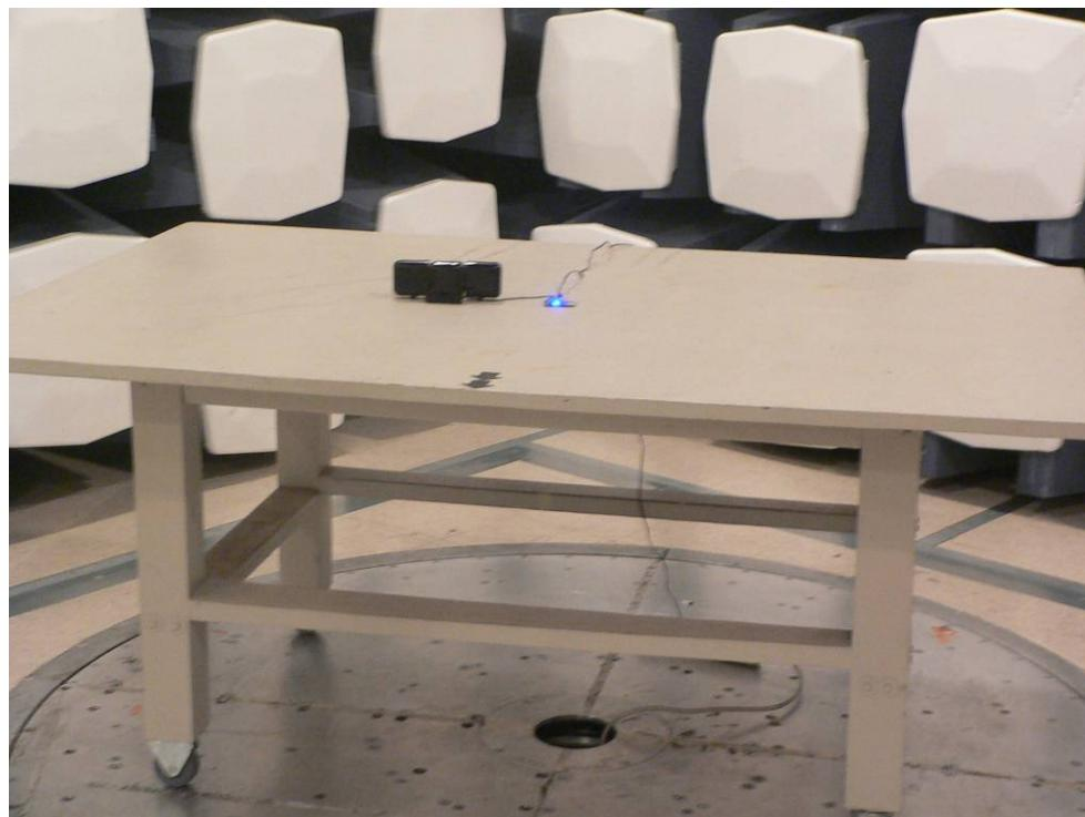
**16.4 Transmitter Radiated Spurious Emissions – Rear View**
