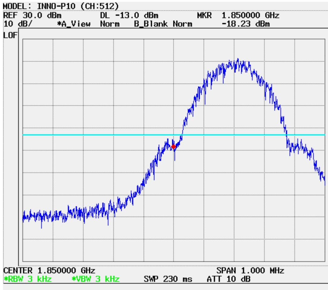
**■ GSM Block Edge GSM1900 (810 CH.)**
