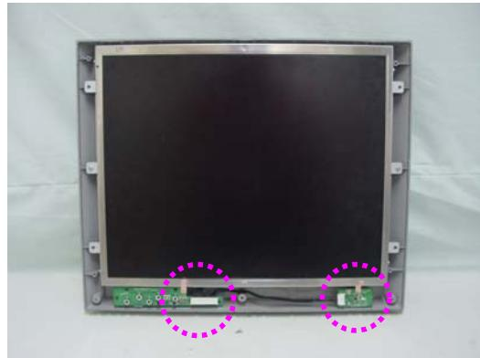
3. Attach a conductive gasket at the LCD's rear panel
