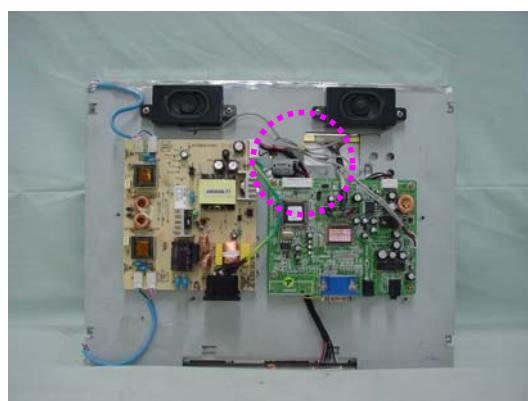
2. Attach a piece of copper foil by bridging it from the LCD panel frame to the OSD board
