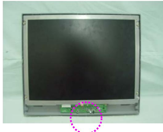
3. Attach a conductive gasket at the LCD's rear panel
