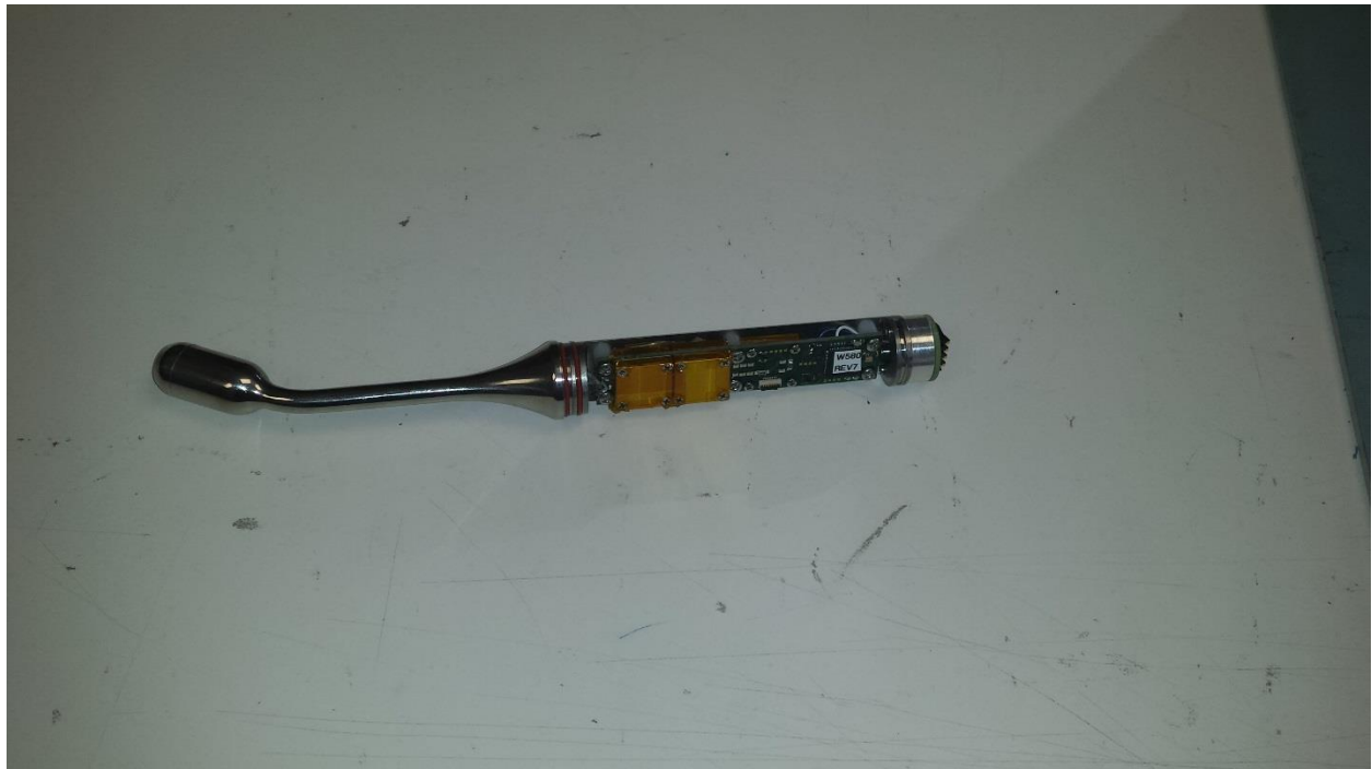
Photograph 2. Wireless Pilot Probe (Transmitter) Assembled
