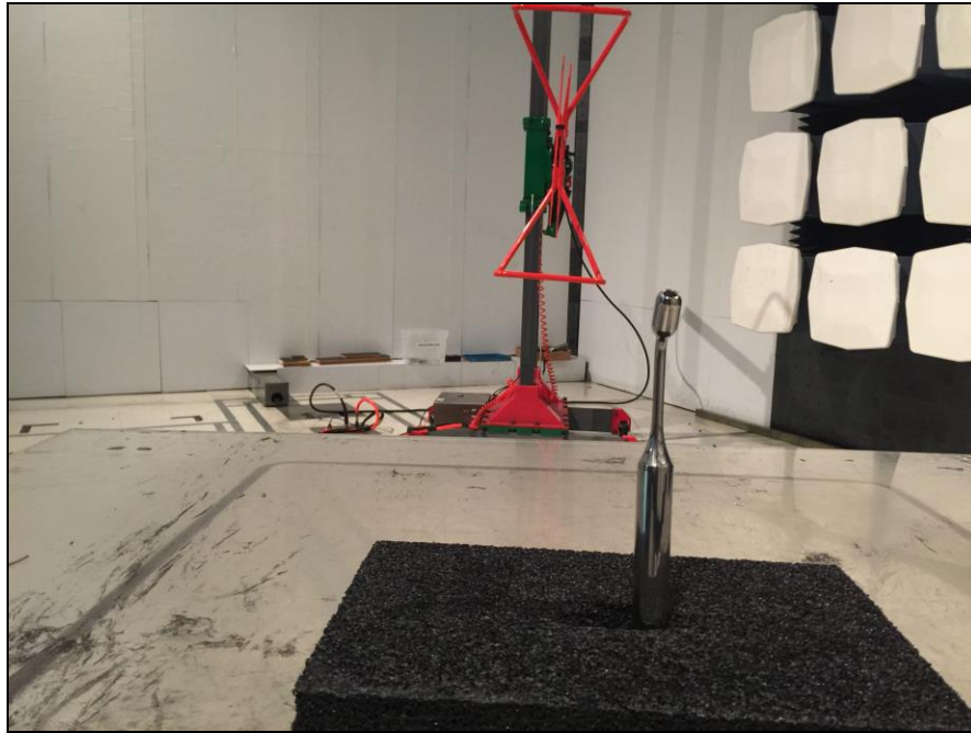
Photograph 1. Radiated Spurious Emissions, Test Setup, Below 1 GHz
