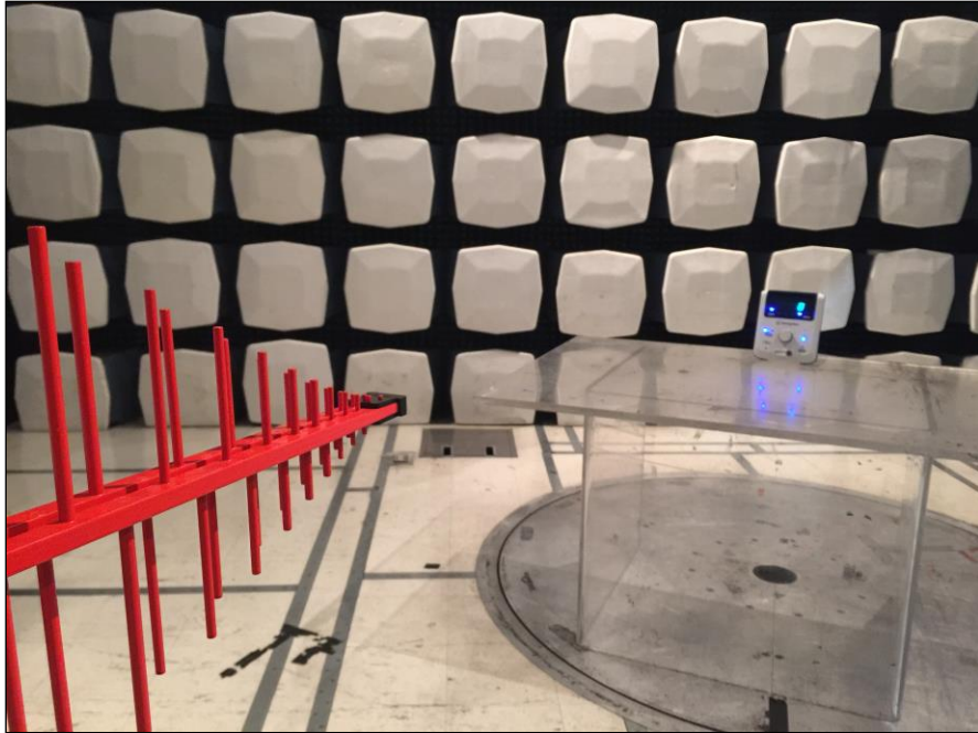
Photograph 1. Radiated Spurious Emissions, Test Setup, Below 1 GHz
