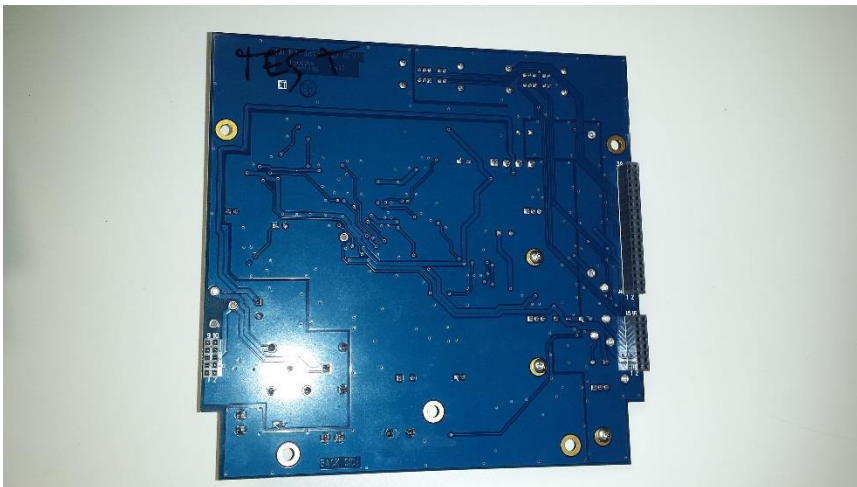
d. Navigator 2.0 System Power Board (Bottom side View)
