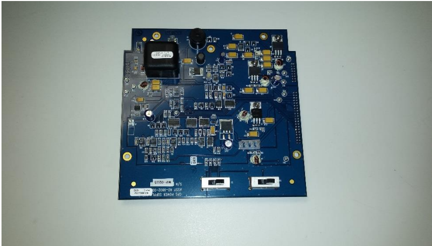
d. Navigator 2.0 System Power Board (Bottom side View)
