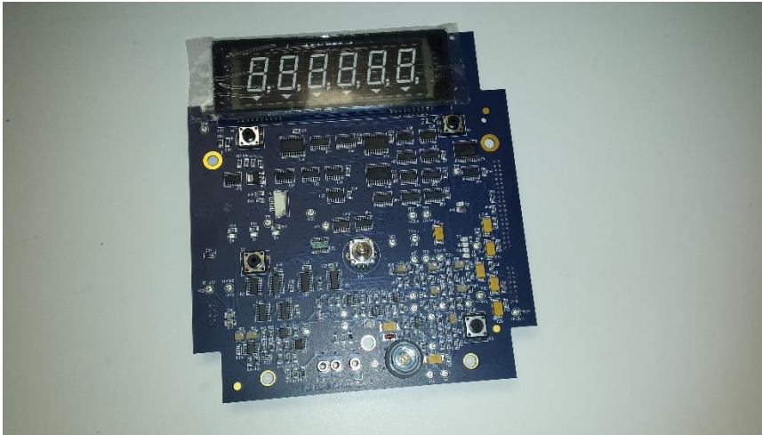
a. Navigator 2.0 System Main Board (Top side View)
