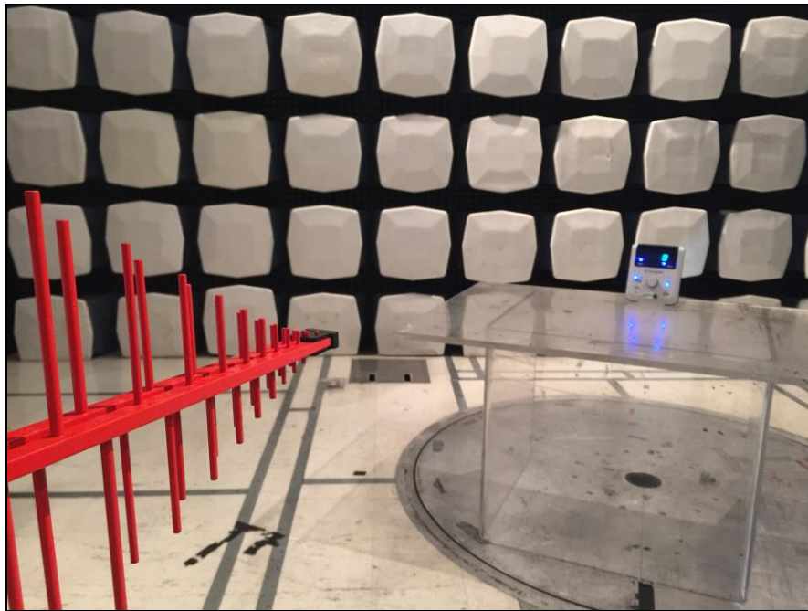
Photograph 1. Radiated Spurious Emissions, Test Setup, Below 1 GHz
