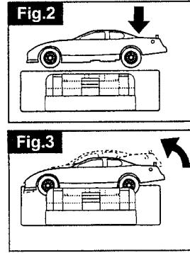
Vehicle has rechargeable Ni-Cd battery. Quick boost charge the Vehicle for around 1 minute by placing the Vehicle on Charger platform correctly. (See diagram Fig. 2) Red LED light **D** indicates that Vehicle is charging. When LED light goes off, charging has been completed. Remove the vehicle from the charging platform as shown in Fig. 3.
