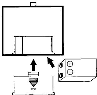
Remove the battery cover on the bottom of the car. Install 2 AA batteries and replace the battery cover.
