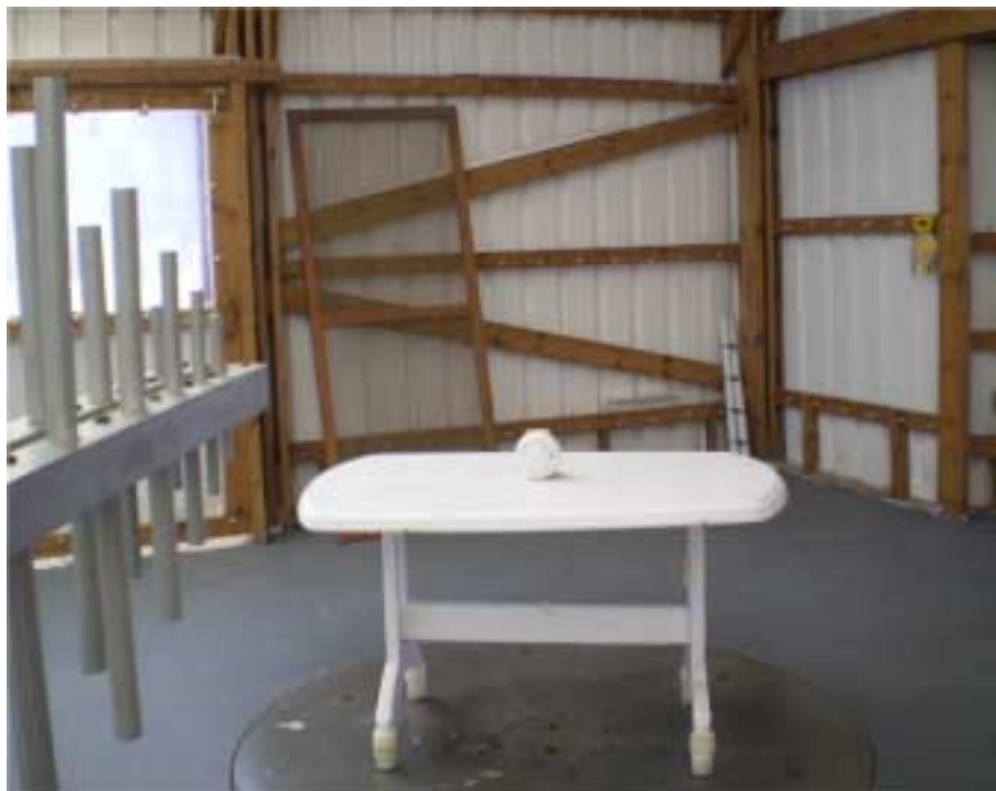
Photograph No.8 Radiated emission field strength measurement setup at the OATS with log-periodic antenna
