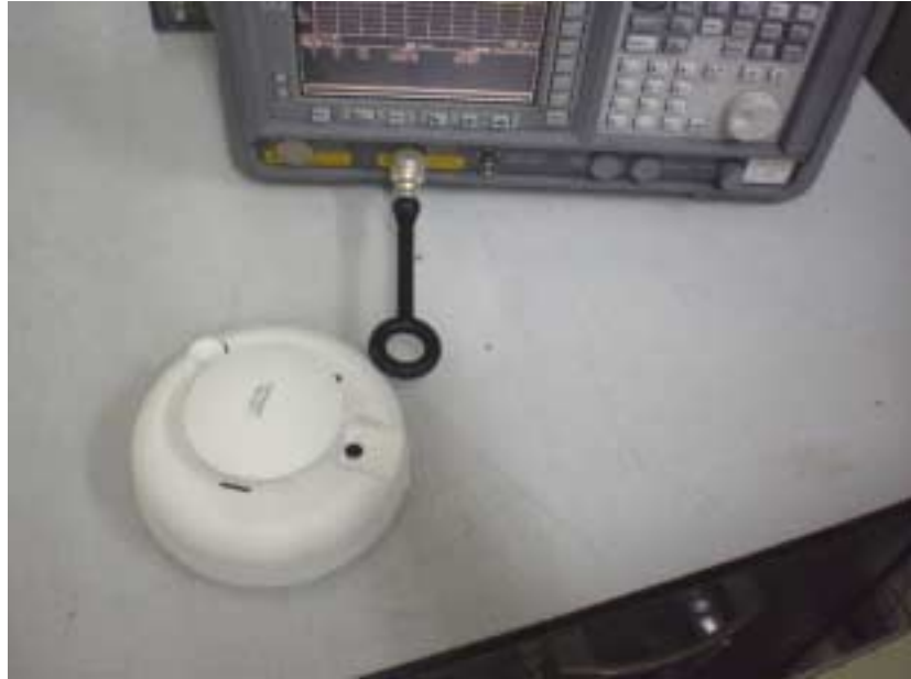
Photograph No.1 Occupied bandwidth measurement setup
