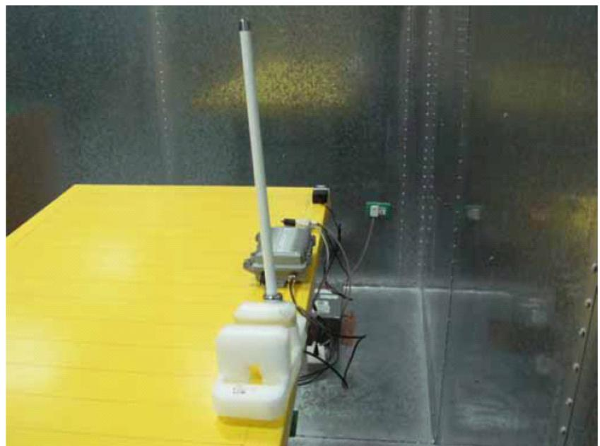
. Photographs of Radiated Emission Test Configuration
