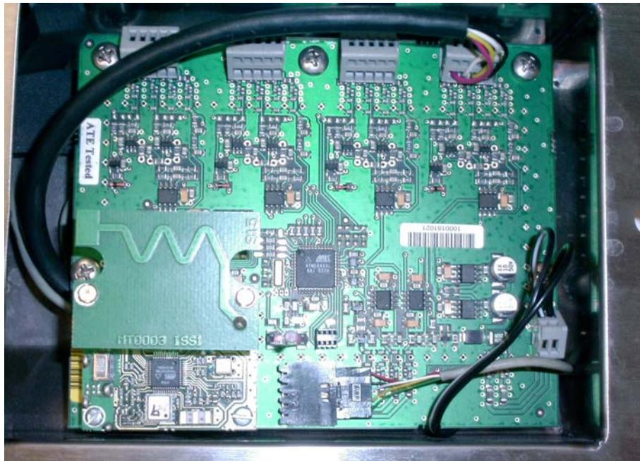
**PHOTOGRAPH OF EUT – *Main Board (Solder Side View)***
