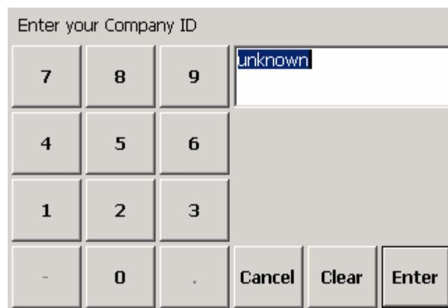
2. Type the Company ID in the data field by touching the numeric keys on the keypad. Touch the **Clear** button if you wish to clear the data field and start over.
