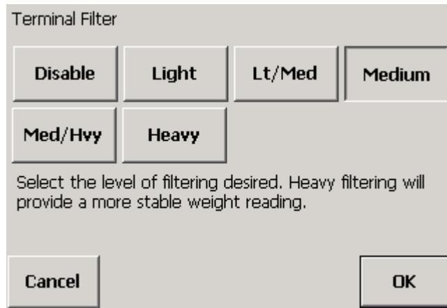
2. Touch a button to disable filtering or to select a filtering level (Light, Lt/Med, Medium, Med/Hvy, or Heavy).
