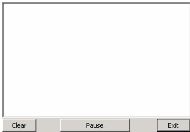
2. Touch the **Pause** button to stop the system from displaying new entries so that you can read the log.
