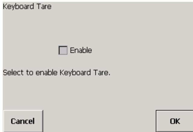
2. Touch the check box to place a check mark in it (enabling the function) or to remove a check mark (disabling the function).
