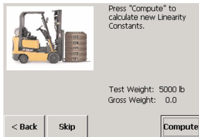
11. Touch the **Compute** button to calculate the new linearity constants.
