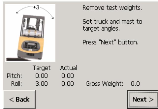
20. Remove the test weight from the scale.
