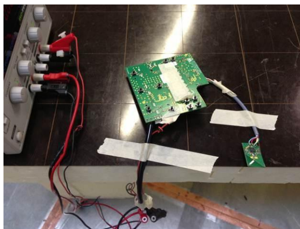
Conducted emission test setup
