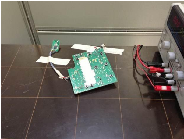
Conducted emission test setup
