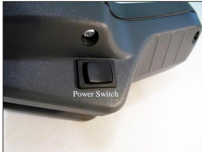
The DP180 rocker power switch has three positions. The middle position is OFF. The end rocker positions are both ON except one provides an additional backlight for the display in low light conditions. Upon first turning the unit ON, the LCD displays the message "Ready". A tag present in the field during power-up will not be processed or displayed upon power-up. It is important to power the unit ON and observe the "Ready" message prior to introducing a tag into the field.
