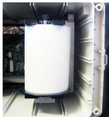
On the upper right side of the roll is the printer release button. Push this button up towards the top of the system, and pull the paper roll towards you to open the printer.
