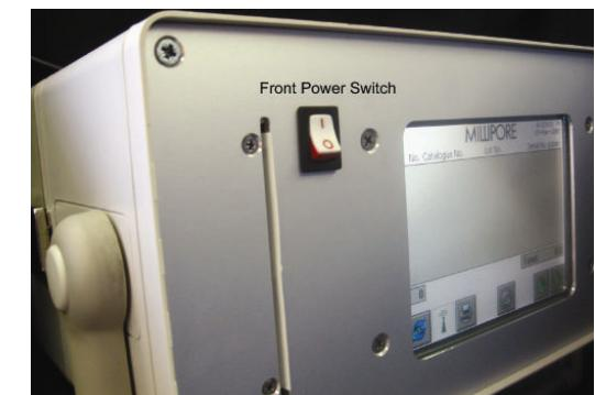
Once the master switch is powered ON, locate the power switch on the front panel of the system and power it ON by pushing the switch towards the top of the system.
