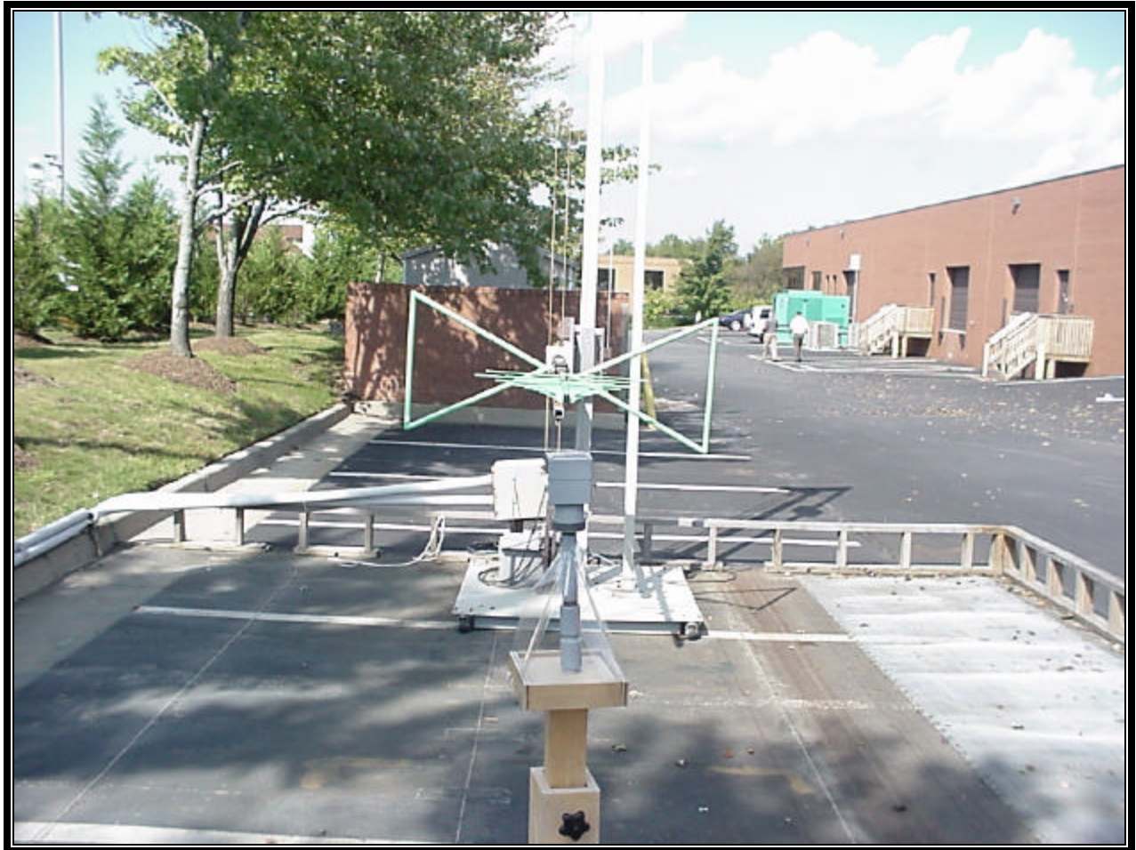
PHOTOGRAPH 3: iTLM-1 WITH WHIP ANTENNA FRONT – RADIATED TESTING
