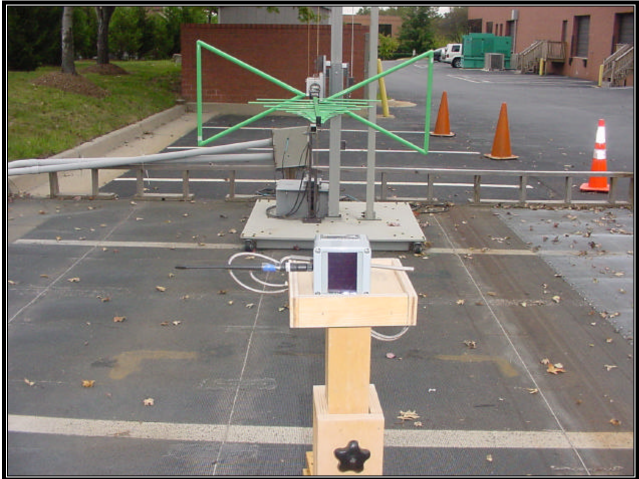
PHOTOGRAPH7: iWPM-T FRONT – RADIATED TESTING
