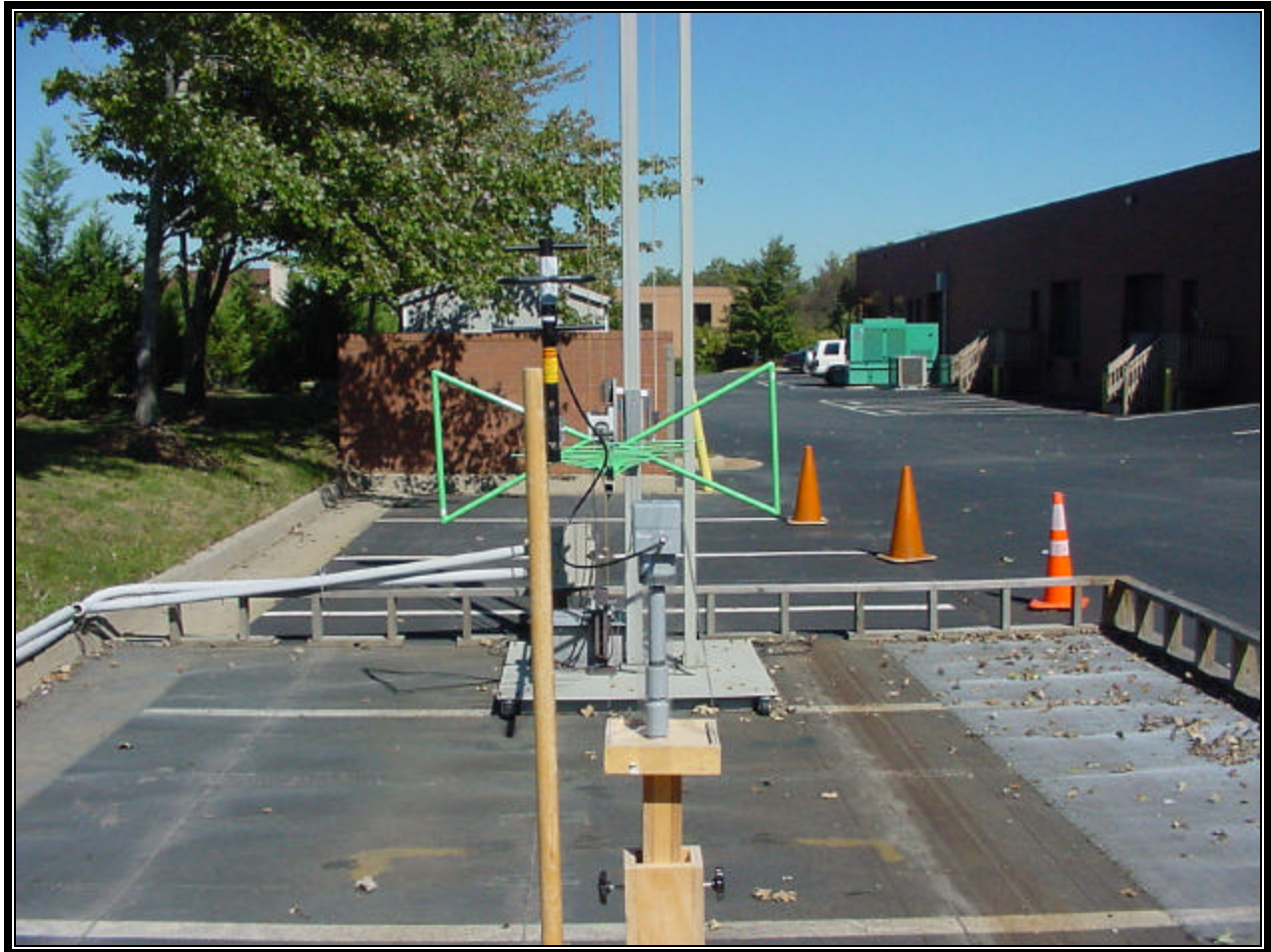
PHOTOGRAPH 6: iTLM-1 WITH YAGI FRONT – RADIATED TESTING
