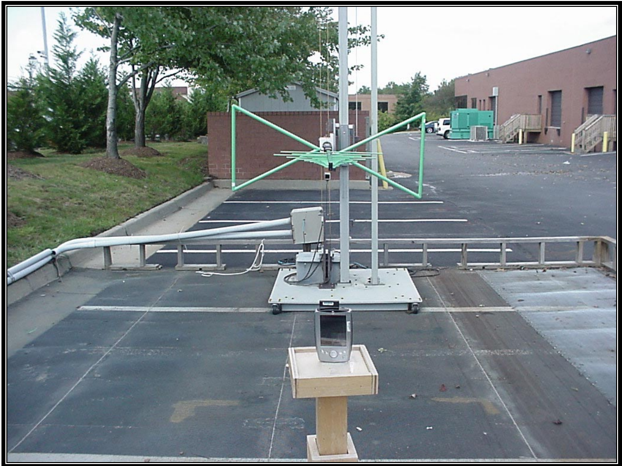
PHOTOGRAPH 1: iCFR FRONT – RADIATED TESTING
