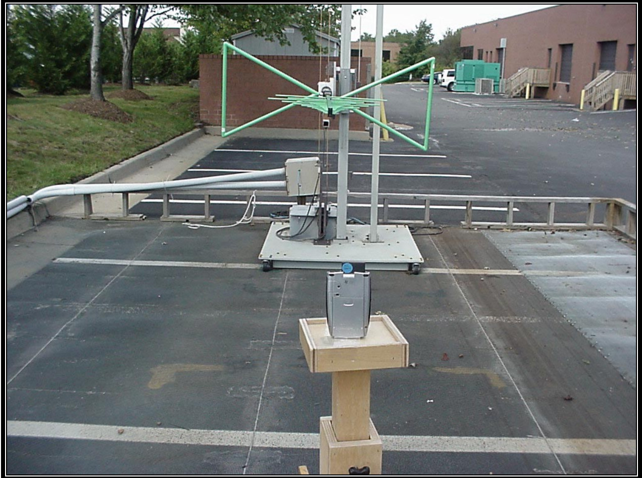
PHOTOGRAPH 2: iCFR REAR – RADIATED TESTING
