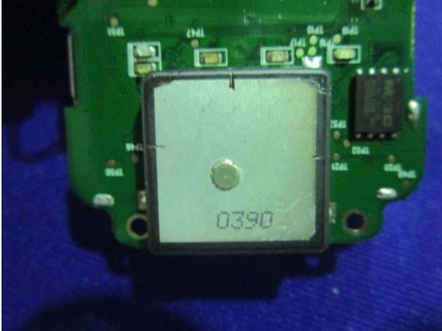
EUT –GPS Antenna View
