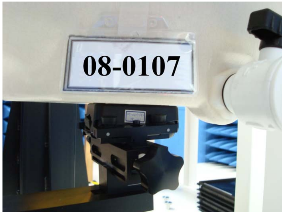
Figure 23. Body SAR Test Setup (Flat Section) _ EUT Bottom with Belt Clip
