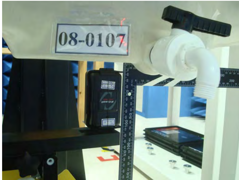
Figure 24. Body SAR Test Setup (Flat Section) _ EUT Tip (Ant. Side) to Phantom 15mm space
