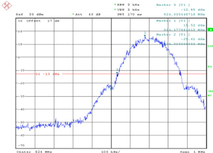
**Band Edge emission GSM Channel high: (GMSK)**
