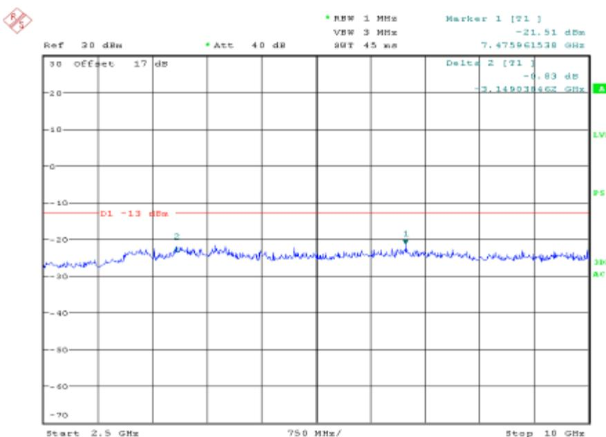
**Band Edge emission GSM Channel Low: (GMSK)**
