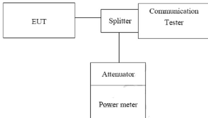
Measurement Setup for testing on Antenna connector.
