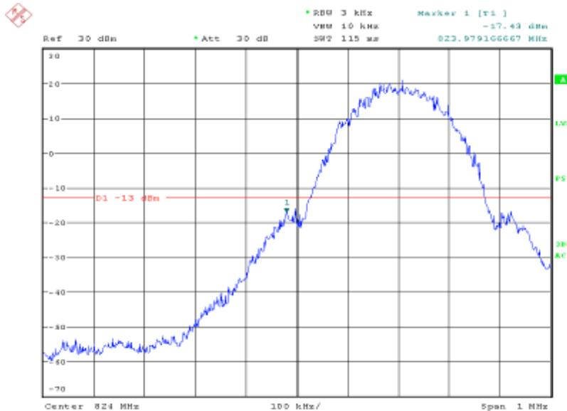
**Band Edge emission GSM Channel High: (8-PSK)**
