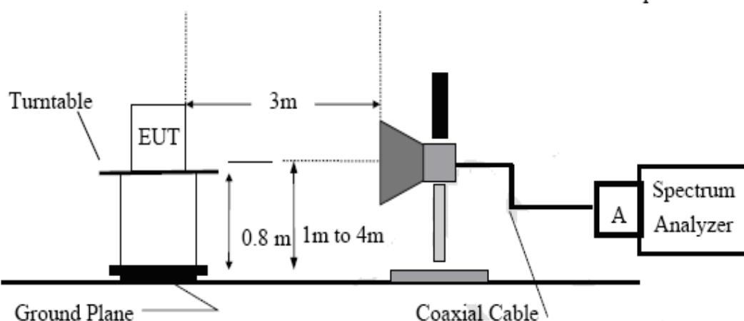
**(C) Substituted Method Test setup:**
