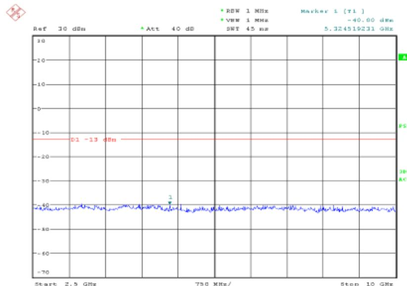
**Band Edge emission GSM Channel Low: (8-PSK)**
