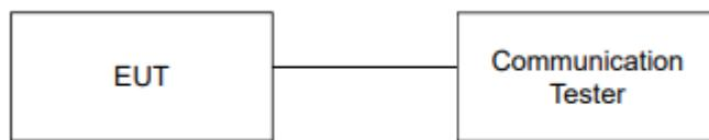
*Note: Measurement setup for testing on Antenna connector*
