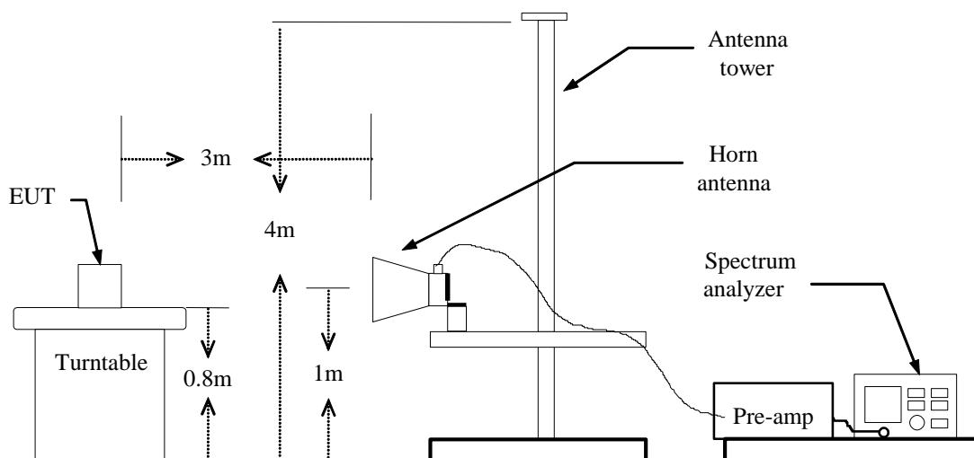
**For Substituted Method Test Set-UP**
