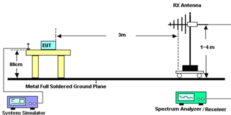
For radiated test from 1GHz to 18GHz
