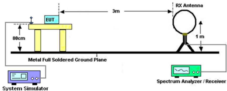
For radiated test from 30MHz to 1GHz
