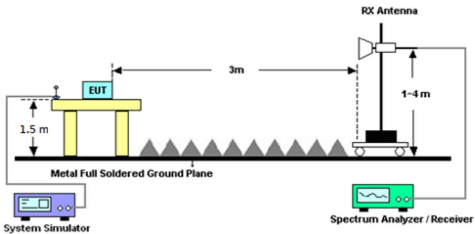
For radiated test above 18GHz
