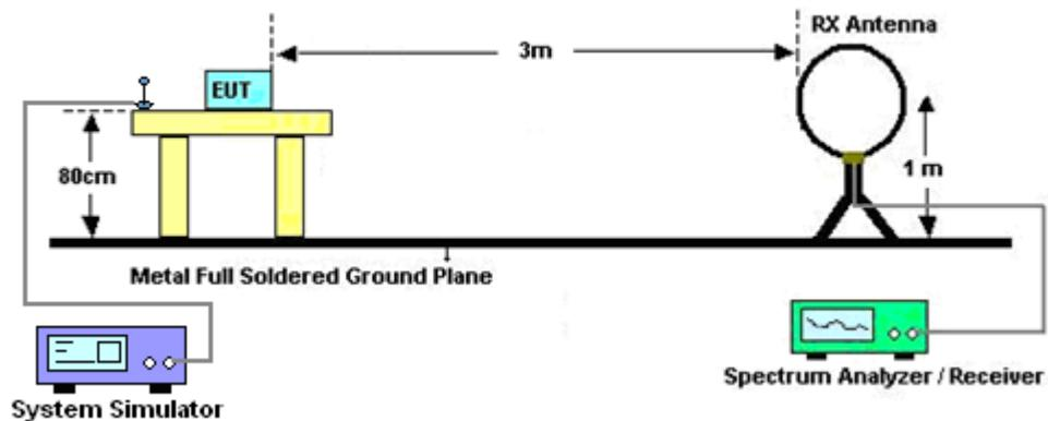
For radiated test from 30MHz to 1GHz
