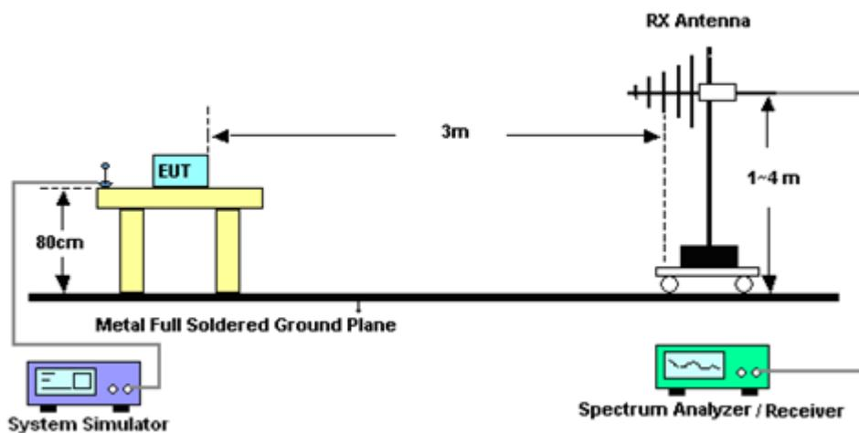
For radiated emissions from 1GHz to 18GHz
