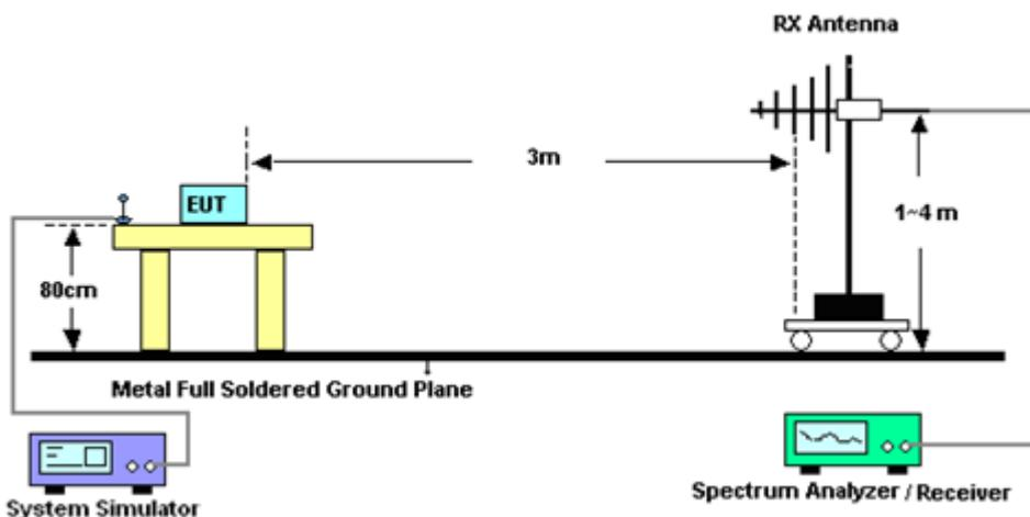
For radiated emissions from 1GHz to 18GHz
