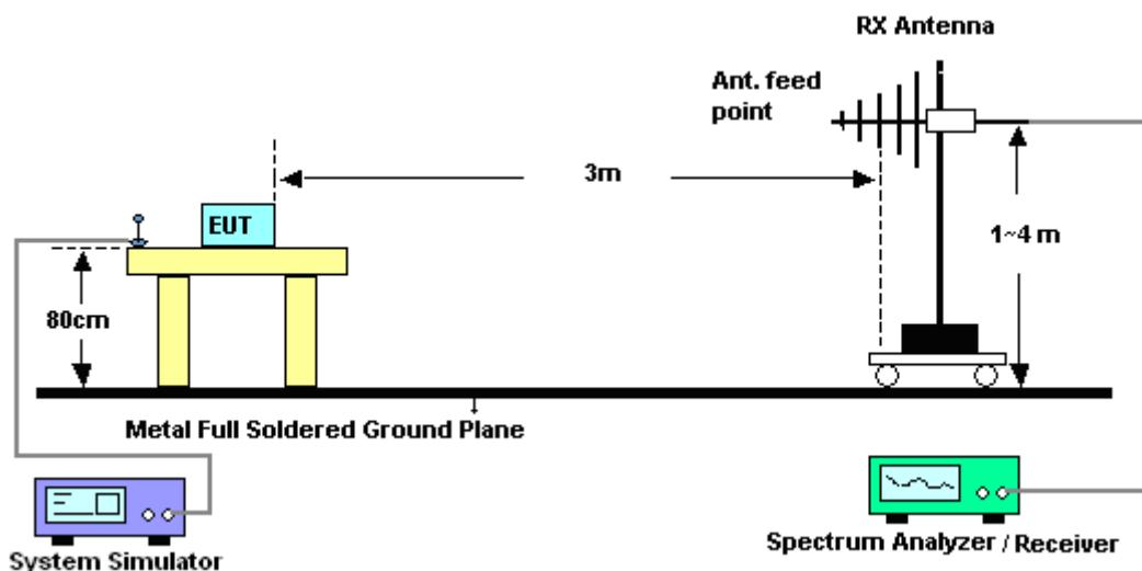
**For radiated test above 1GHz**
