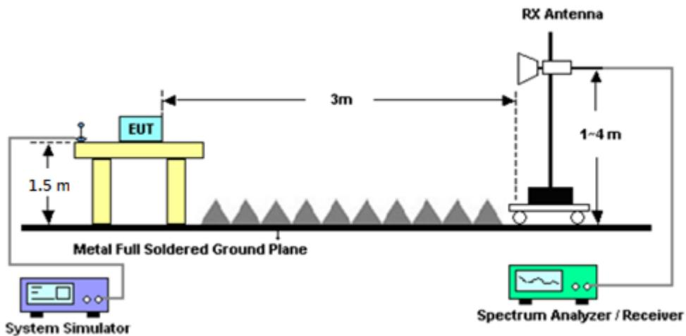
For radiated test above 18GHz
