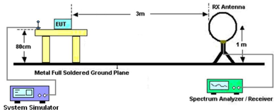
For radiated test from 30MHz to 1GHz
