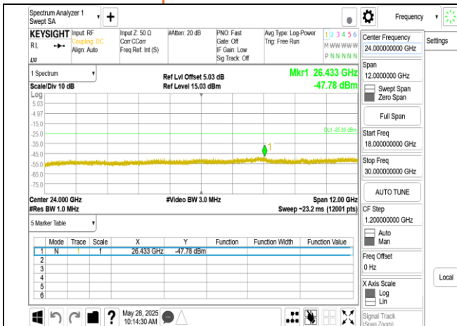
Band38 10MHz DFT s OFDM SCS30kHz BPSK RB1 1 CH515000 upper 18G
