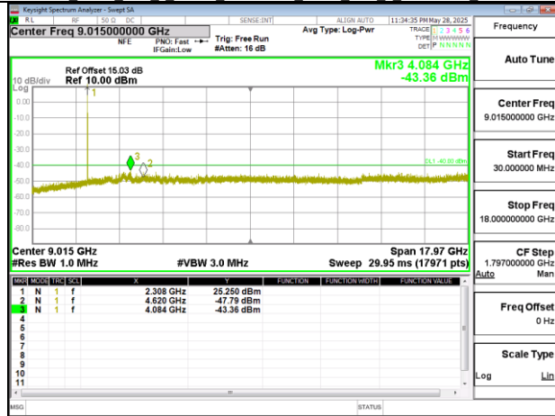
Band30 5MHz DFT s OFDM SCS15kHz BPSK RB1 1 CH462000 below 18G
