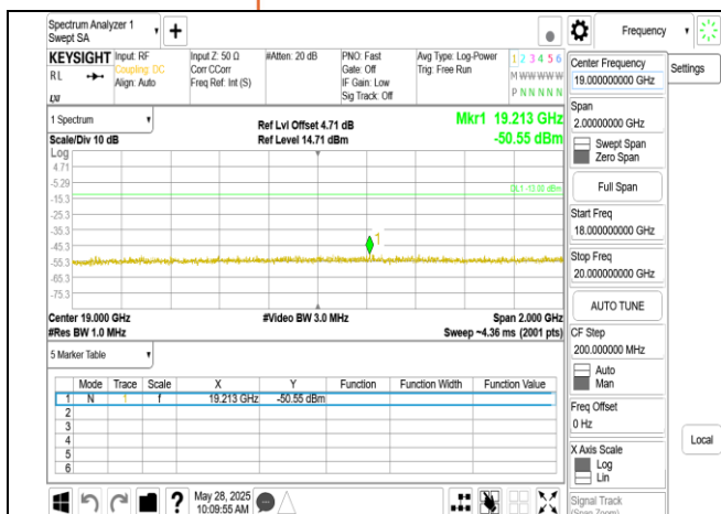
Band25 15MHz DFT s OFDM SCS15kHz BPSK RB1_1 CH371500 upper 18G
