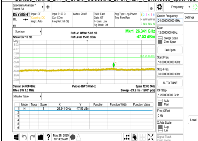
Band38 10MHz DFT s OFDM SCS30kHz BPSK RB1 1 CH519000 upper 18G
