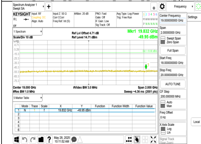
Band25 20MHz DFT s OFDM SCS15kHz BPSK RB1_1 CH376500 upper 18G
