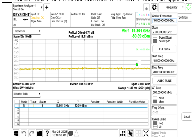
Band25 15MHz DFT s OFDM SCS15kHz BPSK RB1_1 CH376500 upper 18G
