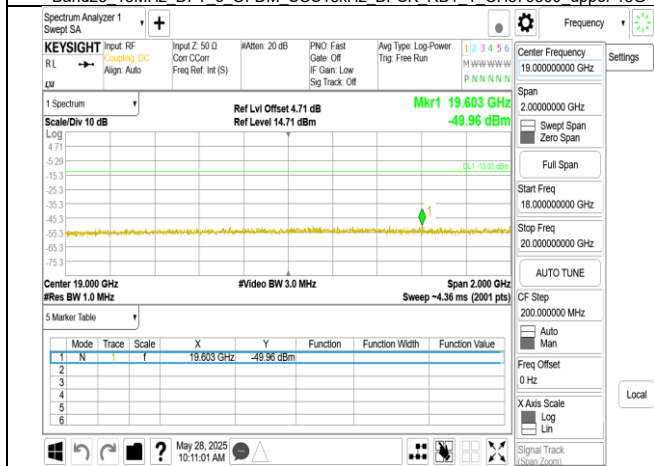
Band25 15MHz DFT s OFDM SCS15kHz BPSK RB1_1 CH381500 upper 18G
