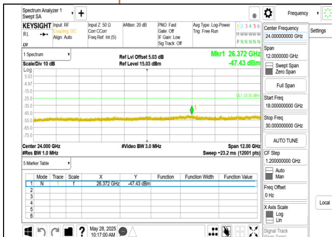
Band38 20MHz DFT s OFDM SCS30kHz BPSK RB1_1 CH516000 upper 18G
