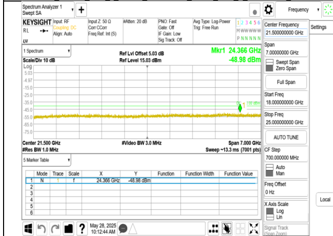
Band30 5MHz DFT s OFDM SCS15kHz BPSK RB1 1 CH461500 upper 18G
