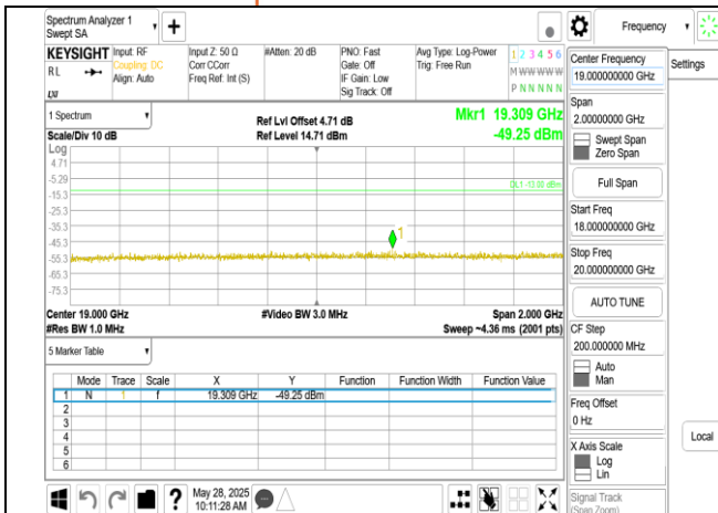
Band25 20MHz DFT s OFDM SCS15kHz BPSK RB1_1 CH372000 upper 18G
