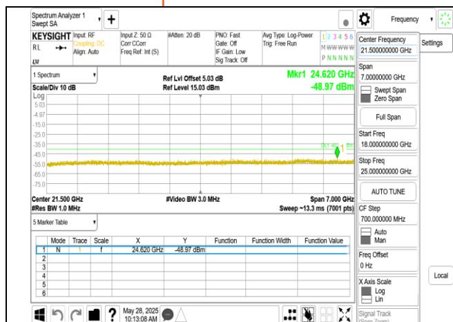
Band30 5MHz DFT s OFDM SCS15kHz BPSK RB1 1 CH462000 upper 18G
