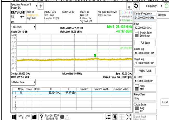
Band38 10MHz DFT s OFDM SCS30kHz BPSK RB1 1 CH523000 upper 18G
