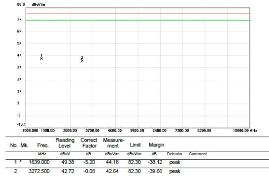
Test Mode : LTE Band 26\_TX CH26740\_5M
