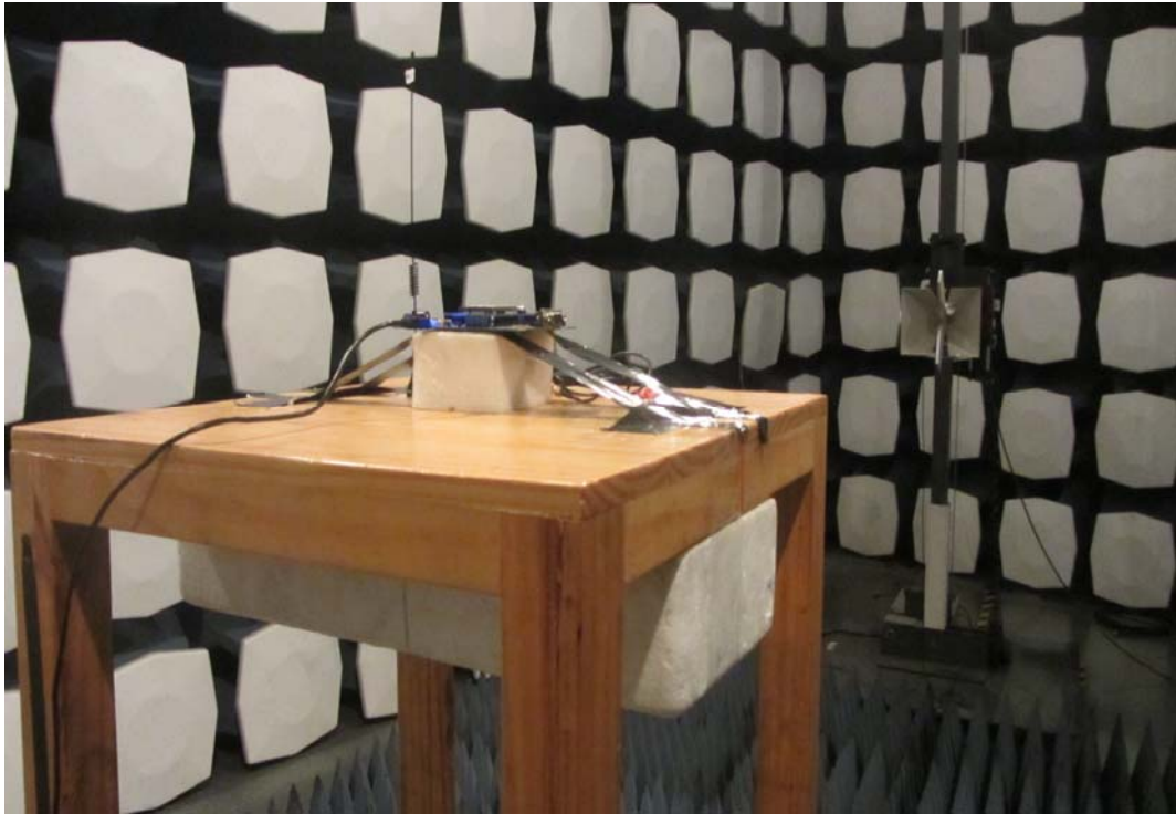
Picture 2: Radiated Spurious Emissions Test setup
