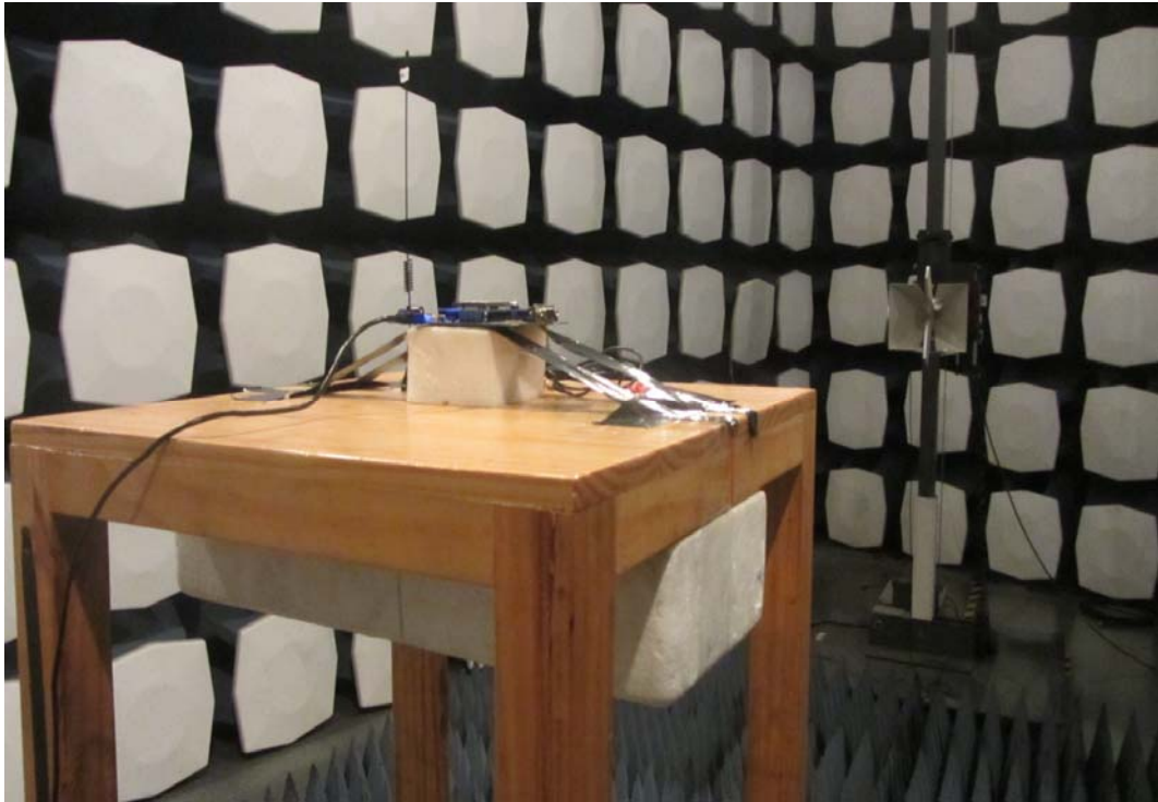
Picture 2: Radiated Spurious Emissions Test setup
