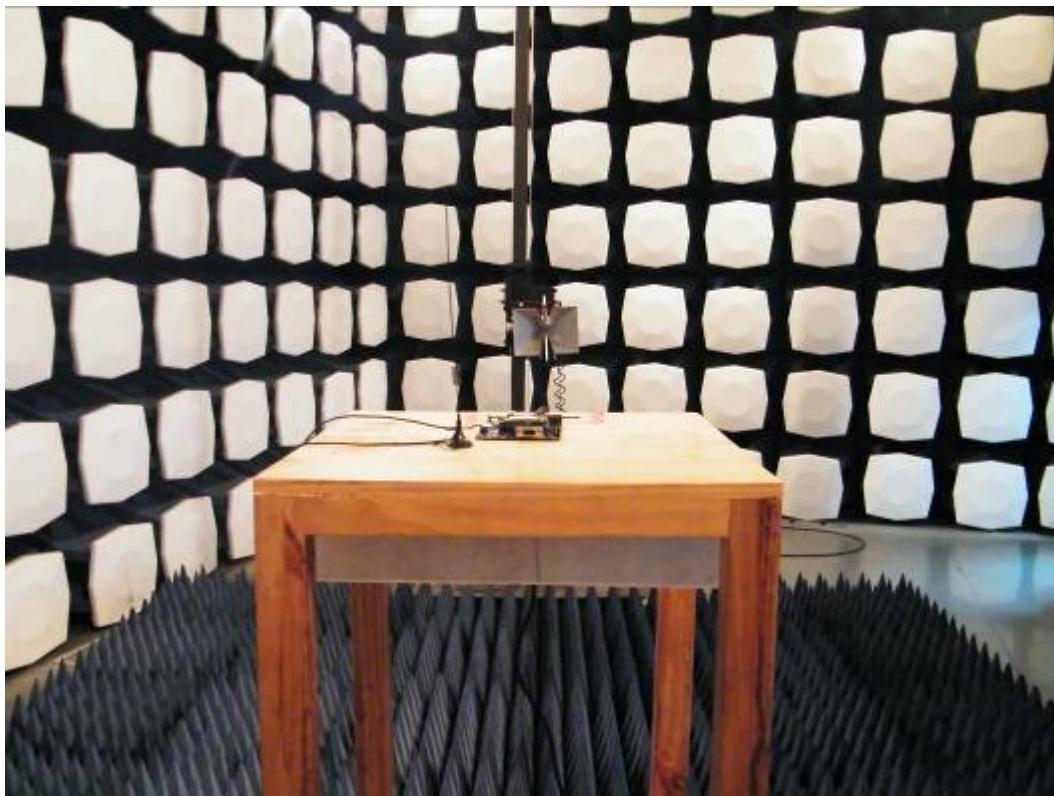
Picture 2: Radiated Spurious Emissions Test setup
