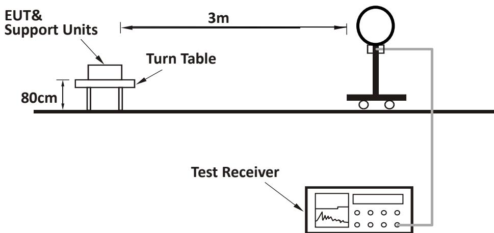
**For Radiated emission 30MHz to 1GHz:**
