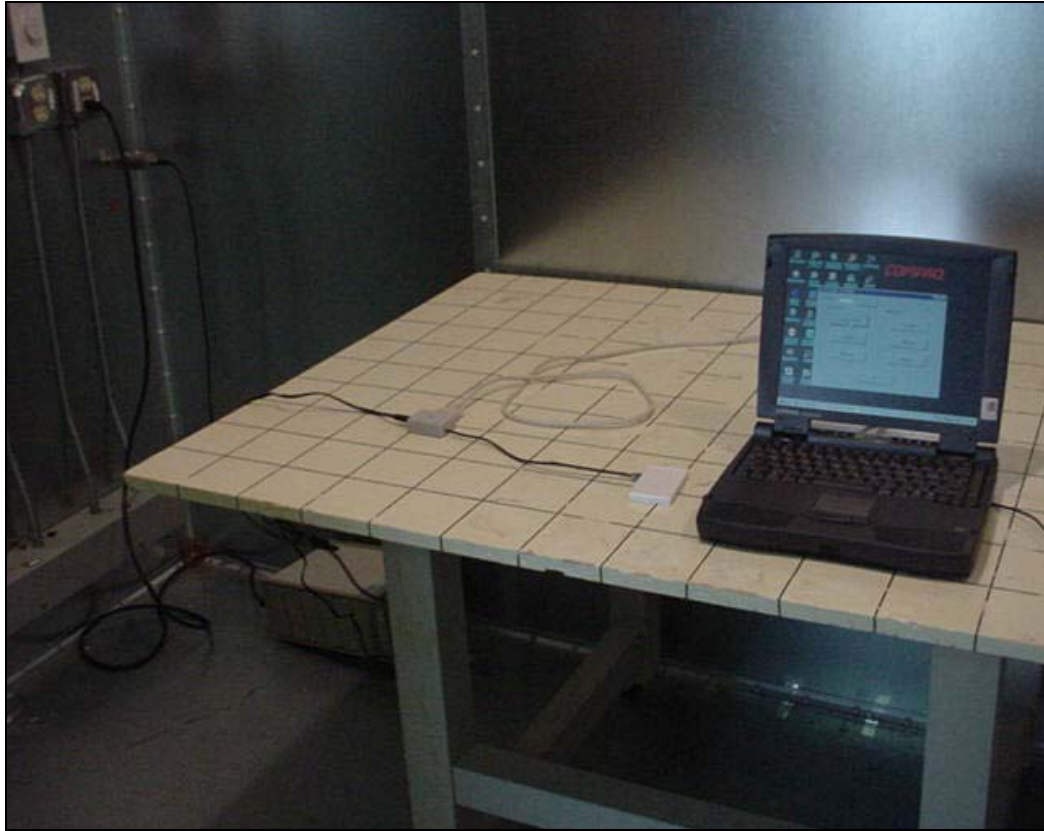
View of the EUT during Conducted Emissions Testing
