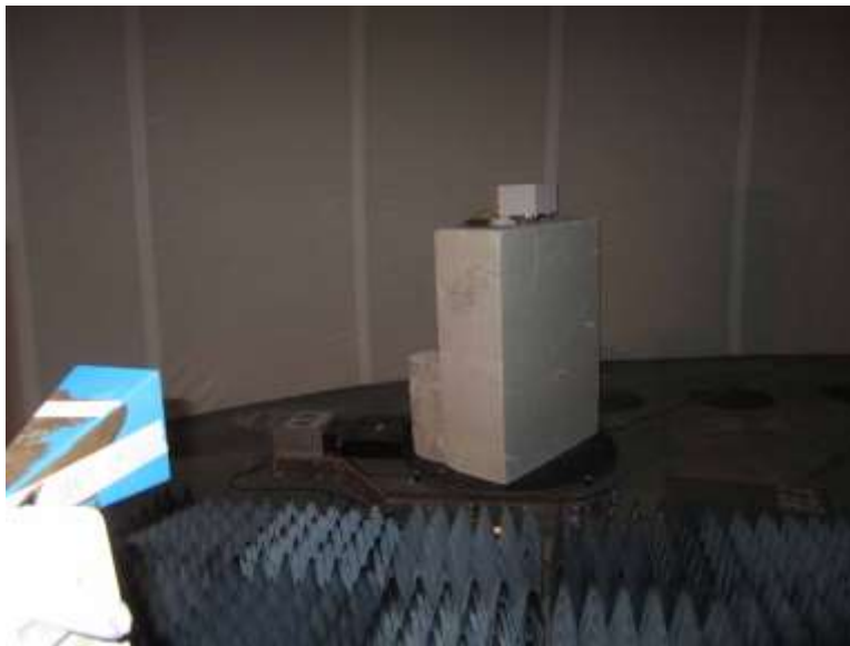
13dBi-Hex-26.5-40GHz, Cone placement
