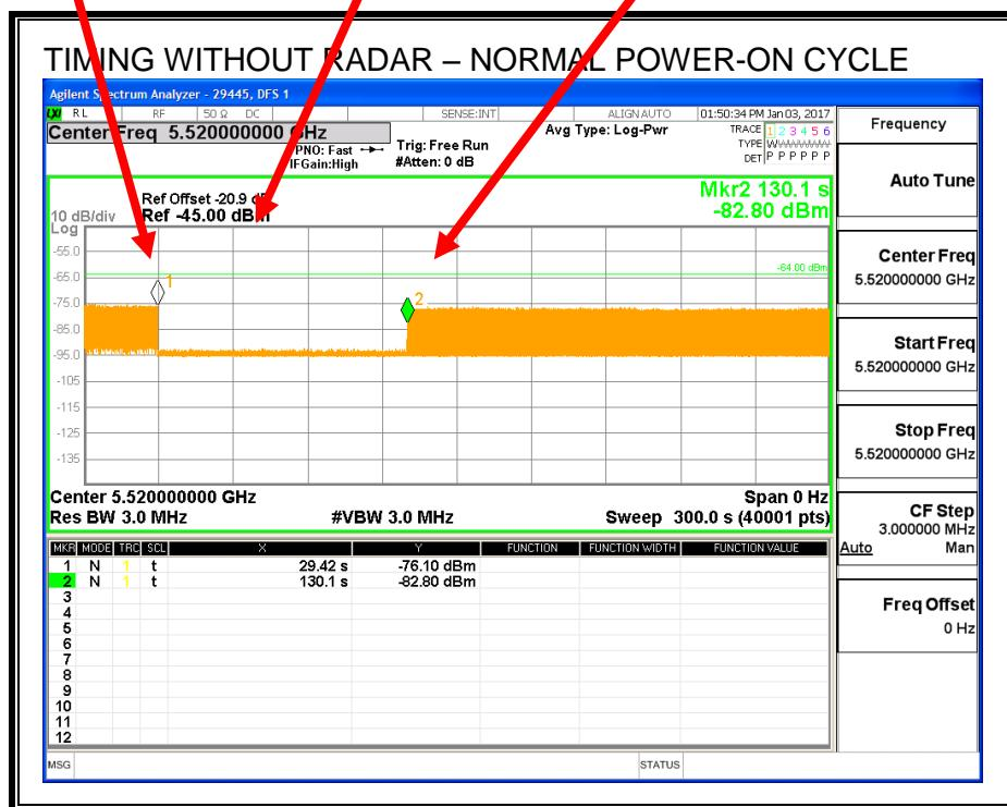
Transmissions begin on channel after completion of the initial power-up cycle and the CAC.
