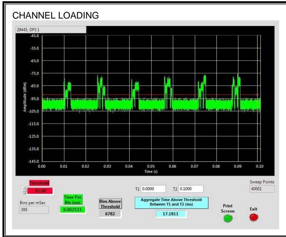
The level of traffic loading on the channel by the EUT is 17.18%
