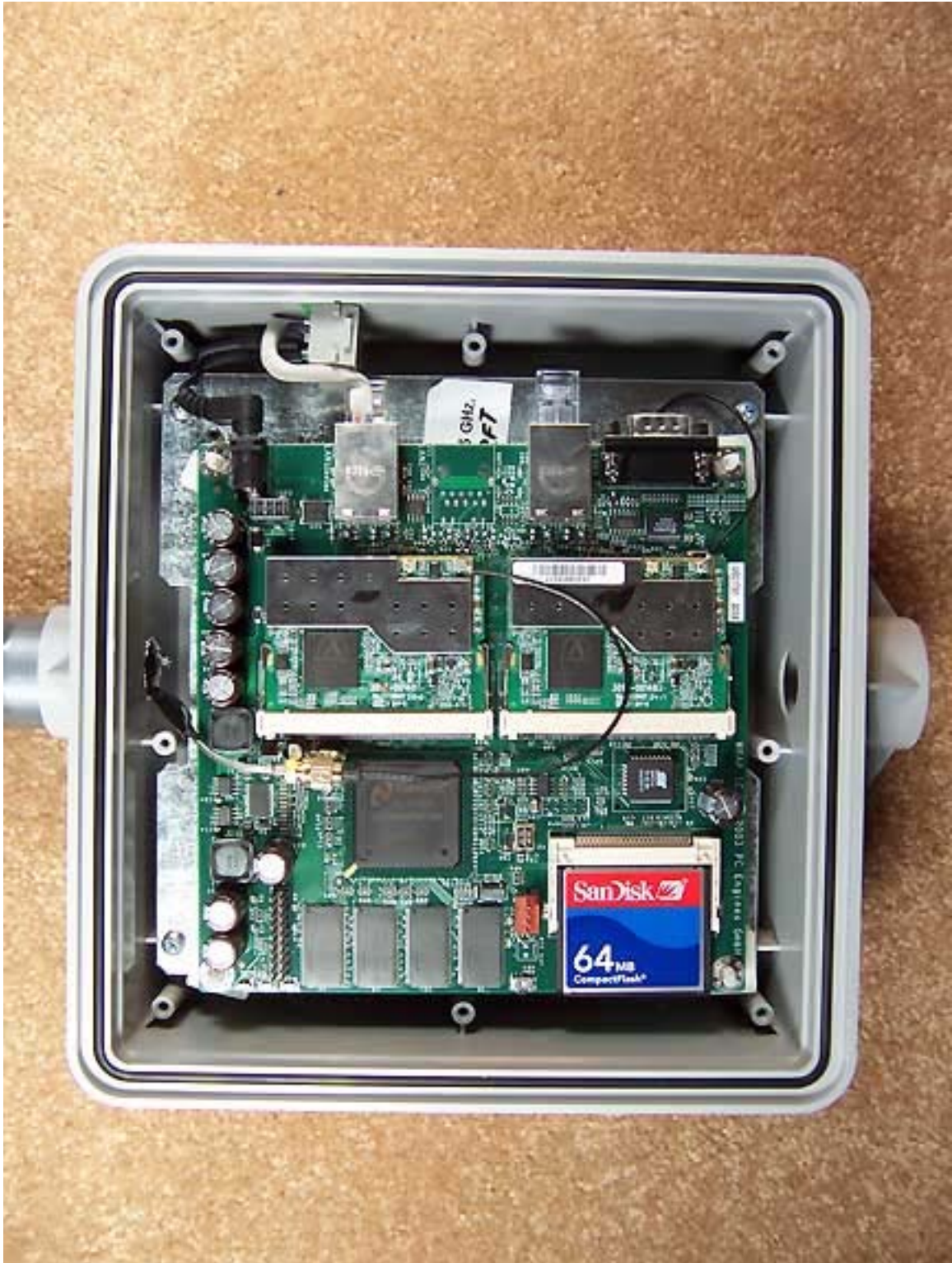
Relay Internal PCEngines
