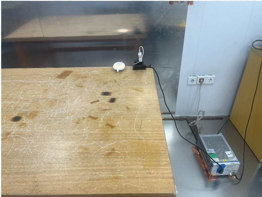
Photo of Setup for Radiated Emission (30MHz~1GHz)
