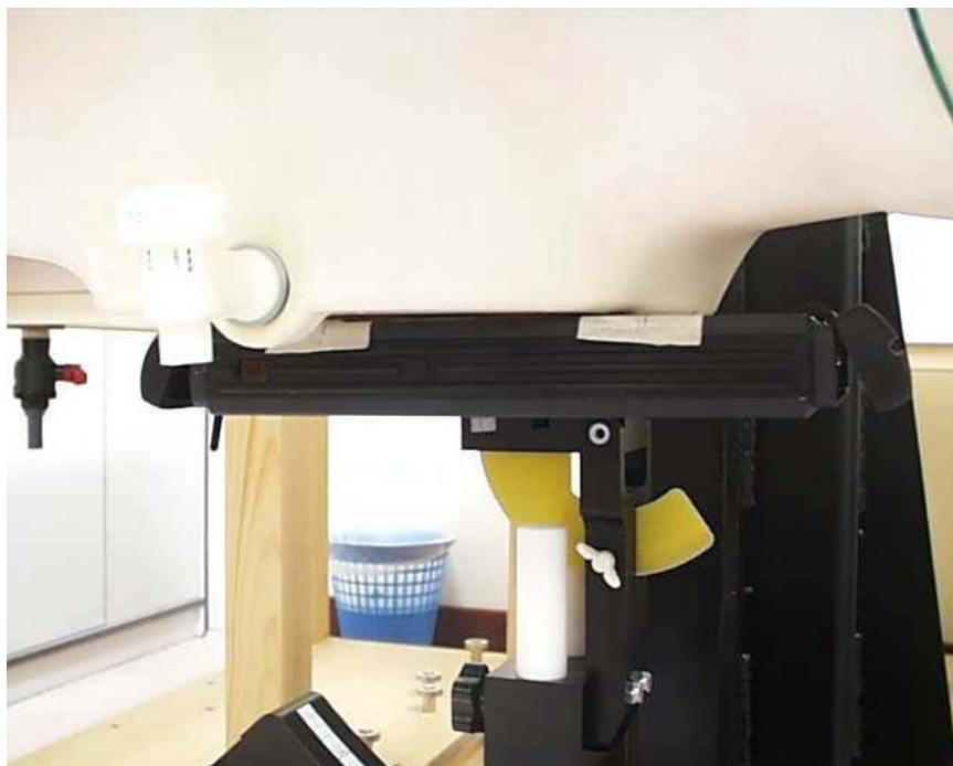
SAR Test Setup At Flat Phantom – Closer Front View (EUT Section A Touched Phantom)
