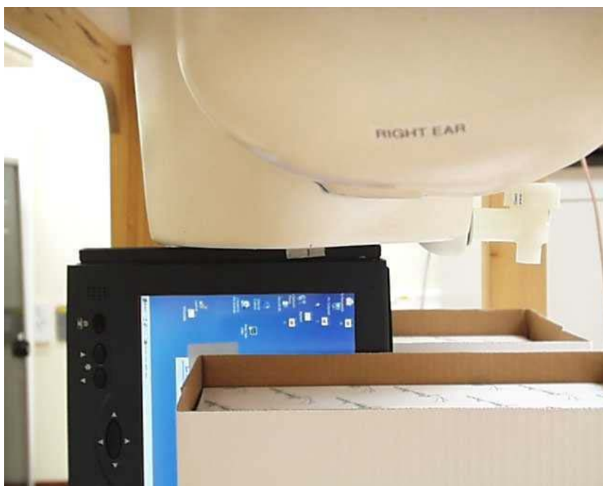
SAR Test Setup At Flat Phantom – Closer Side View (EUT Section E Touched Phantom)
