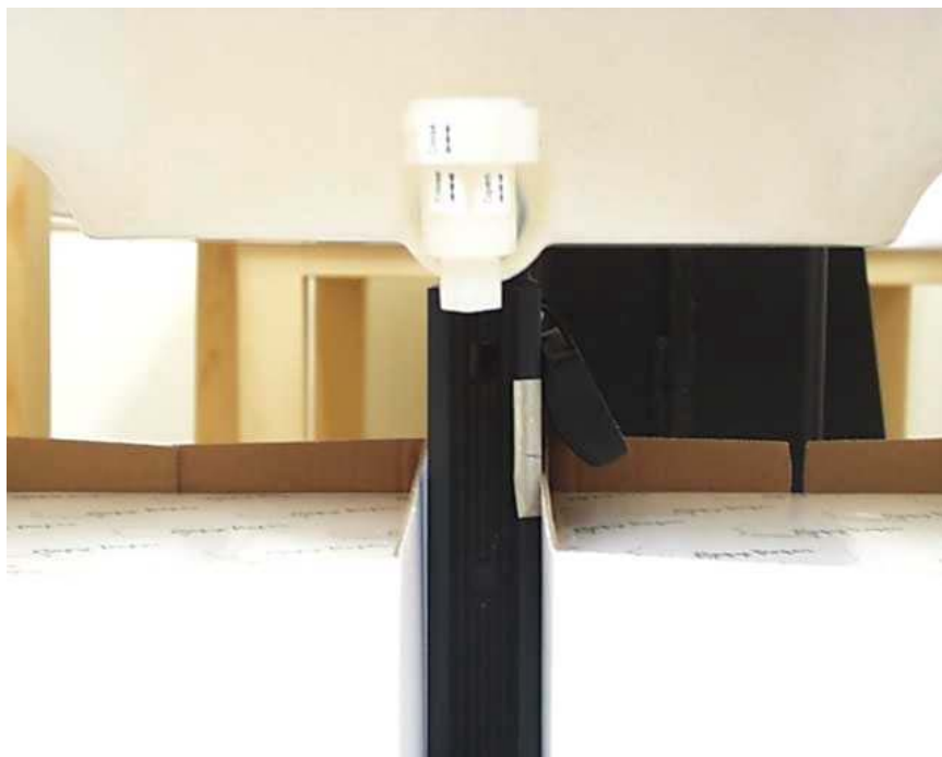
SAR Test Setup At Flat Phantom – Closer Front View (EUT Section E Touched Phantom)
