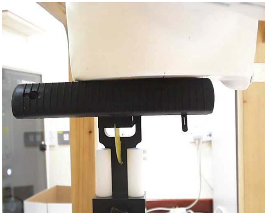
SAR Test Setup At Flat Phantom – Closer Side View (EUT Section A Touched Phantom)
