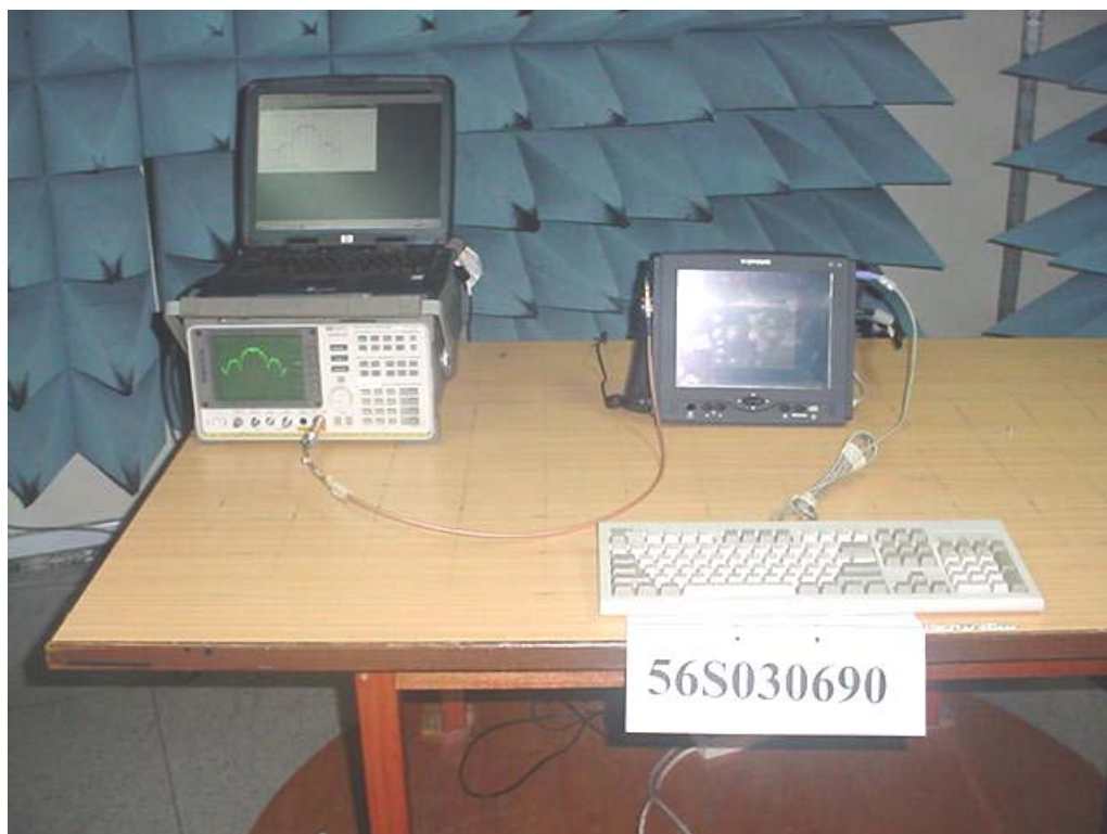
Peak Power Spectral Density Measurement Test Setup
