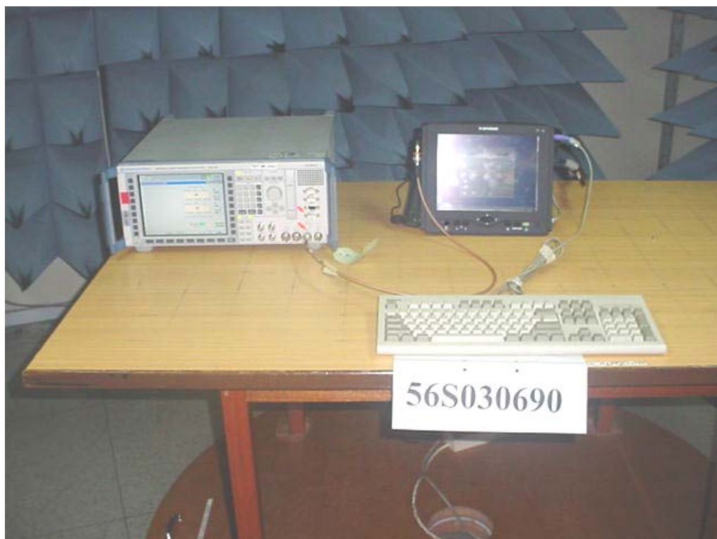
Maximum Peak Power Measurement Test Setup
