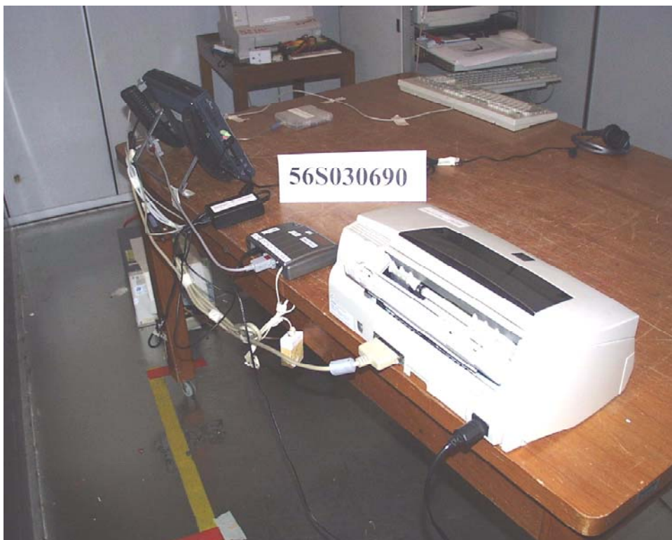
Conducted Emission Setup (Rear View)
