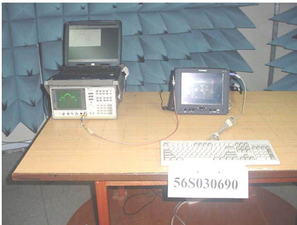
Spectrum Bandwidth Measurement Test Setup
