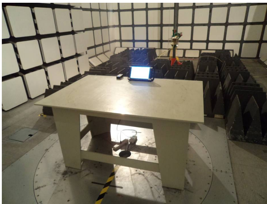
Radiated Emissions – Front View (Above 1GHz)
