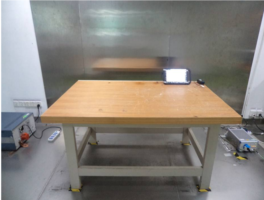
AC Line Conducted Emissions - Front View
